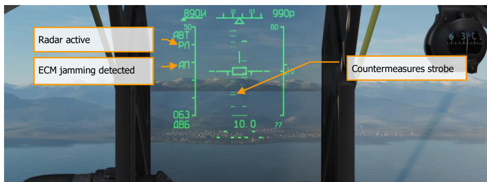
Figure 44: SCAN Mode with jammer strobe
