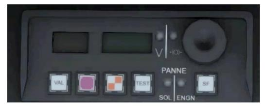
The orange display shows control information regarding warning speeds, while the green display shows signal or line speed information.
