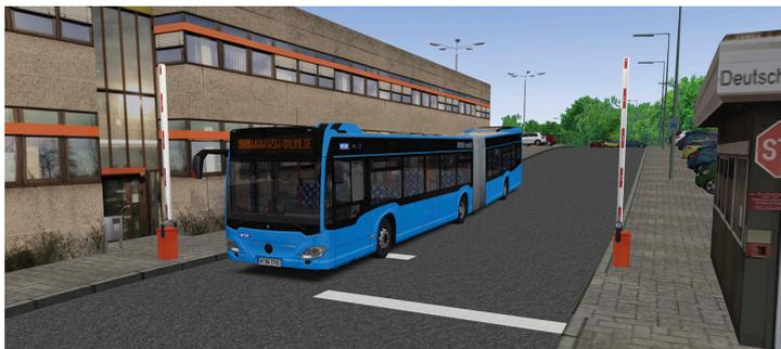
The articulated bus features 3 swing-in doors and a completely low-floor interior. It also has an Euro 6 engine and 4-speed automatic transmission, but no passenger AC.
