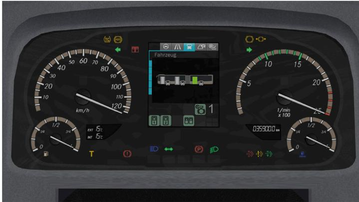
In contrast to the older monochromatic and well-arranged displays, a new small colored display was introduced. There are several check lights scattered over the panel, while some icons are also shown in the display.
