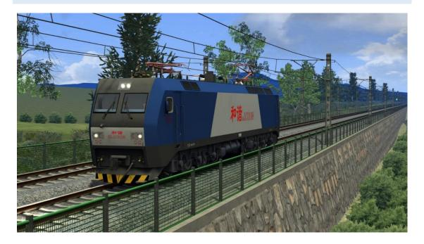
The HXD1C locomotive is a high-power AC drive six-axle electric locomotive with a power of 7200 kW. It was designed with its own set of fully independent intellectual property rights. 90% of its components are made in China. The locomotive's design makes use of nine main technology patents, being the locomotive's assembly, carbody, bogie, traction transformer, traction converter, network control system, traction motor, driving device and brake system.
