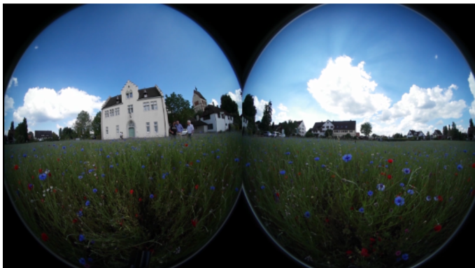
Unstitched video from the two 180° fisheye lenses from a 360° camera
