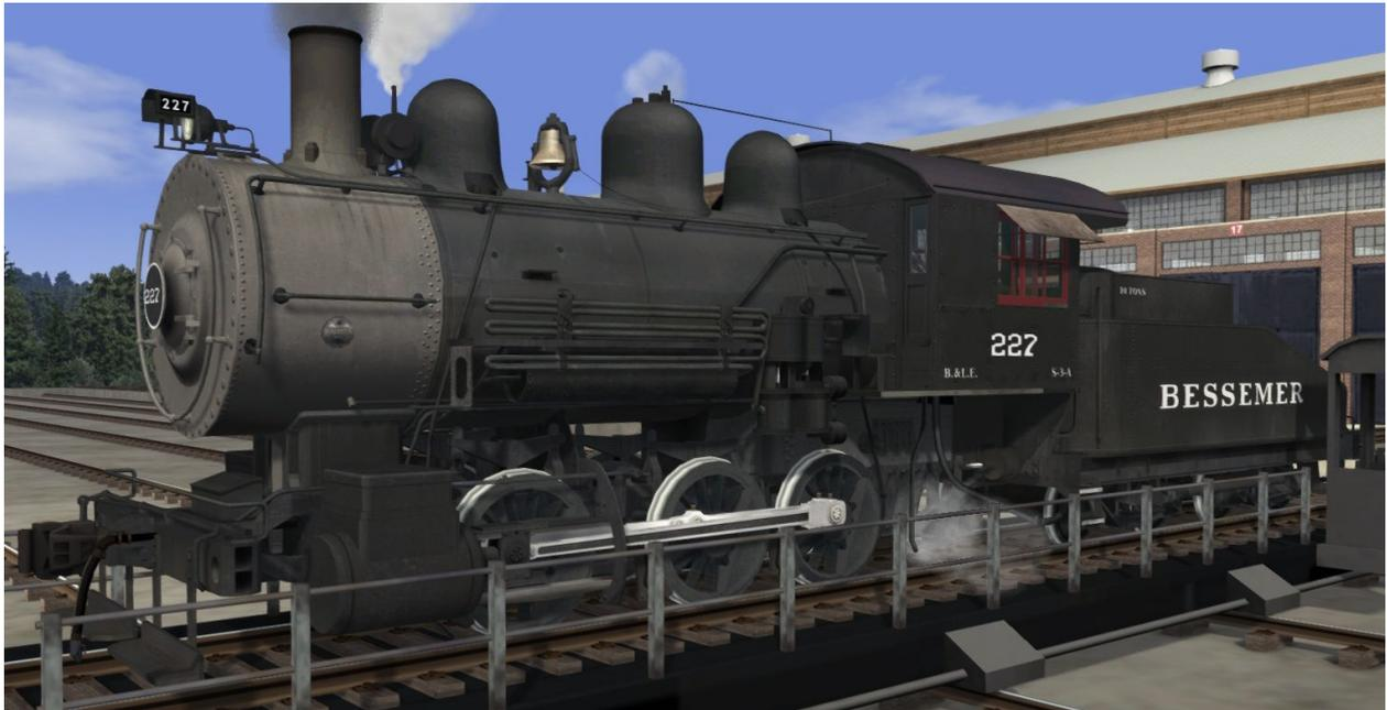
During the turn-of-the-century era, the B&LE owned eleven coal-fired "Six-Coupled" 0-6-0 steam locomotives. The final seven 0-6-0s, modeled here, were built by Baldwin beginning in 1909. They were used primarily for switching duty in the yards, assembling ore and coal trains. Though the Baldwin delivery included a sloped-back tender, a conventional tender is also included for variety.
