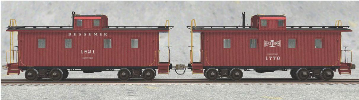
No train of the 1920s is complete without a caboose. This wooden body four-axle caboose, built in the B&LE's own Greenville shops, is a typical example of a caboose from that era.
