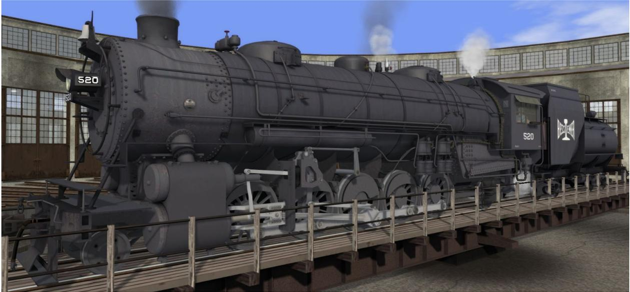
The B&LE owned 25 coal-fired "Santa Fe" 2-10-2 steam locomotives. All were built by Baldwin beginning in 1916, including 19 D-1-A class, as modeled here. These locomotives were designed for tractive power rather than speed, hauling heavily laden ore and coal trains over the full route. The locomotives were equipped with a Street mechanical stoker, and a Vanderbilt-style tender. The "Bessemer" labeled tender is provided in both railhead (shown) and block-lettered formats.
