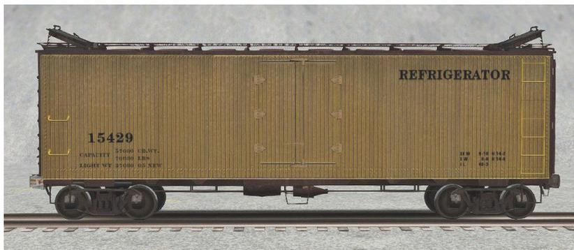
This is a wood-and-steel body icebox refrigerator car, used to transport agricultural produce and other perishables. Blocks of ice can be filled into boxes below the four hatches on the roof, keeping the interior of the insulated car cool for many hours.
