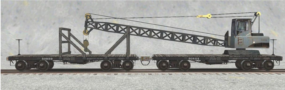
A small maintenance-of-way and wreck crane for lighter duties. Built on top of an old 30 ft flatcar frame and matched with a similarly home-built boom car.
