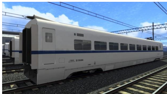
Car No.4: Trailer car with pantograph
