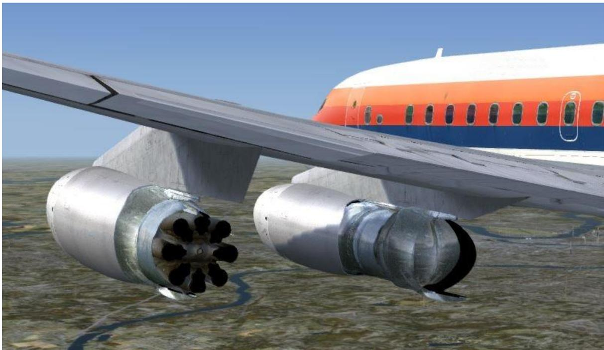
Extend the ejectors for engines 3 and 4 by using the INBD ENG INJECTORS switch on the overhead panel.
