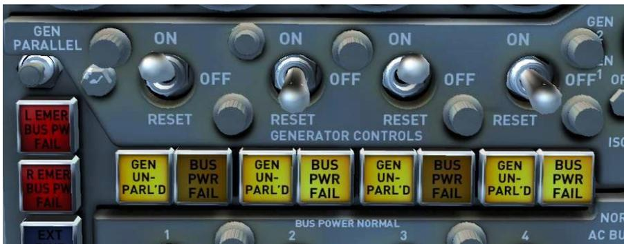
Before moving on from the electrical panel, ensure that the four Bus Power switches are in the **ON** (up) position.
