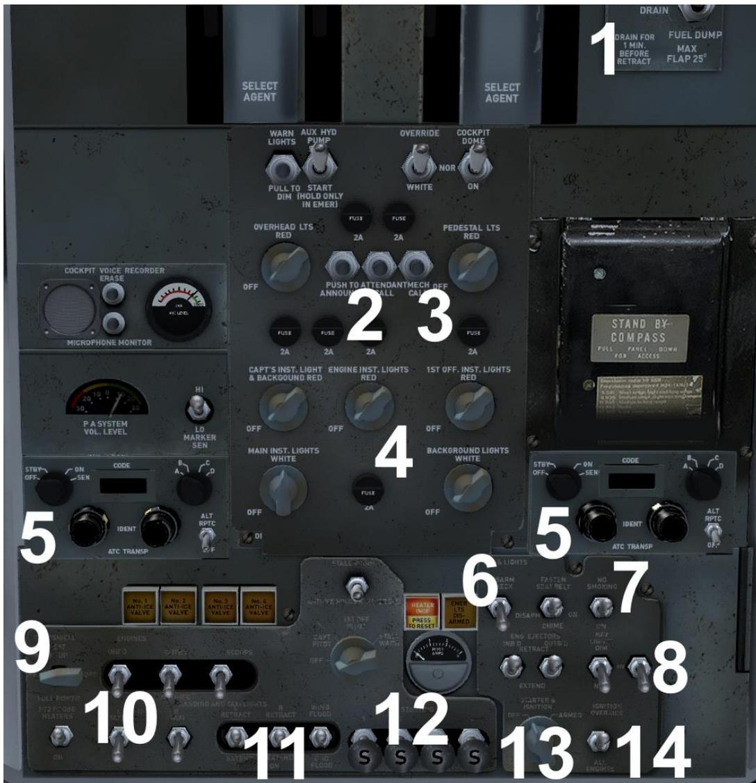
The procedure for engine start requires that you first arm the ignition, followed by the ignition switch, before pressing the starters. You will find that unless you follow this procedure you will not be able to use the starter buttons.
