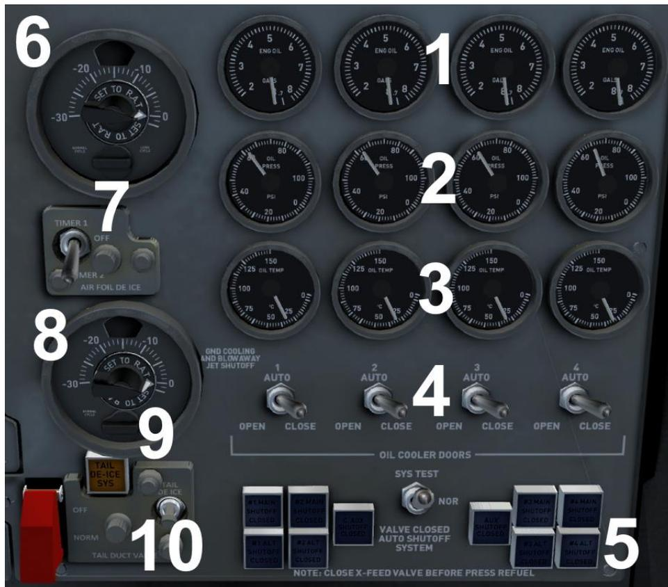
1. Engine oil quantity gauges
