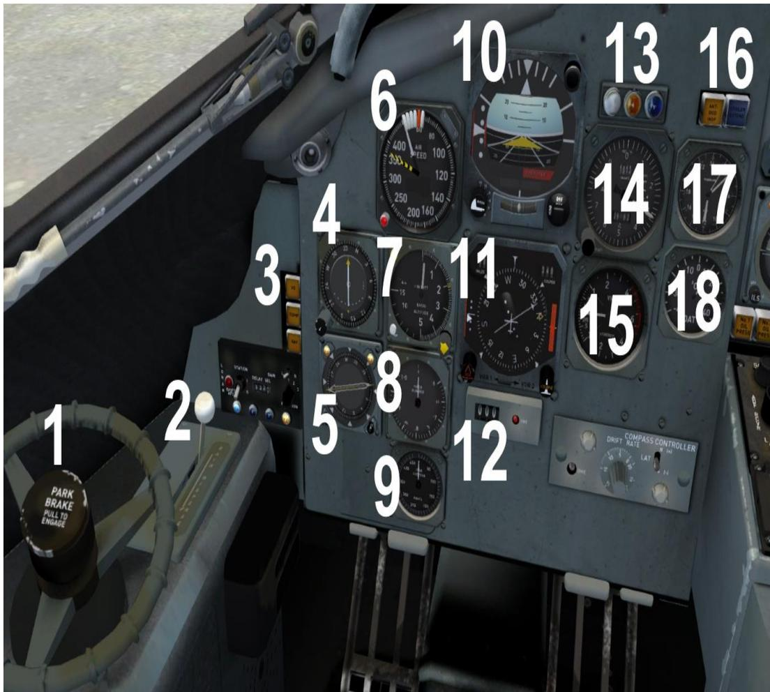
1. Parking brake and nose-wheel steering tiller
