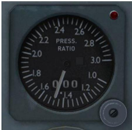
The EPR gauge indicates a power setting for a given engine. This is used in combination with special EPR tables to establish the correct throttle settings for a given cruise altitude and speed. The EPR bugs can be set to the desired thrust reading using left- or right-click (or the mouse-wheel), and the selected setting is indicated in the tumbler window. Throttles can then be adjusted to achieve the desired thrust range.
