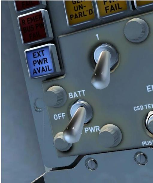
There are four generators, one per engine. No.1 generator is responsible for bringing the power bus online so that avionics and major electrical supplies can be energised. The engine start procedure calls for engine No.3 to be started first, so turn on both the No.1 and No.3 generators.
