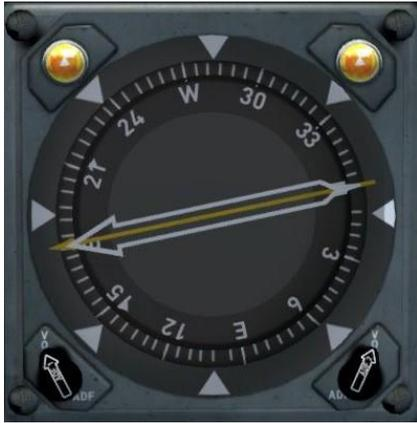
The HSI can be driven either by NAV 1 or NAV 2, depending on the position of the switch at the bottom of the gauge.
