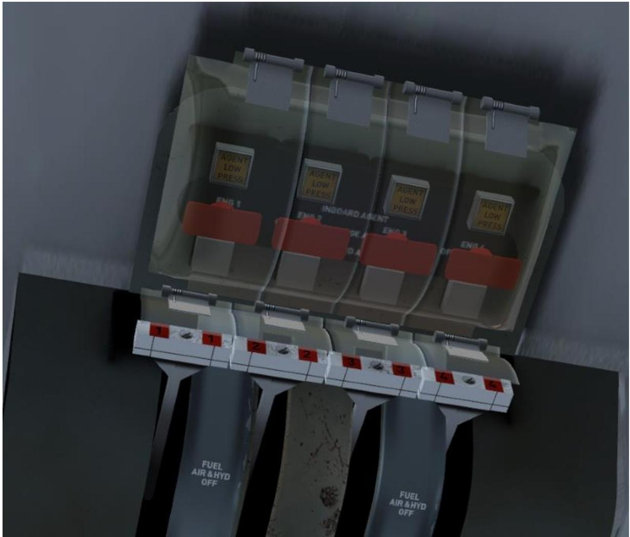
To operate the system, lift the clear perspex cover for the affected engine (1 through 4, left to right). Click on the red lever. The lever will swing down to the discharge position as will the agent/select lever. To reset the system, simply click on the red lever again and close the cover.
