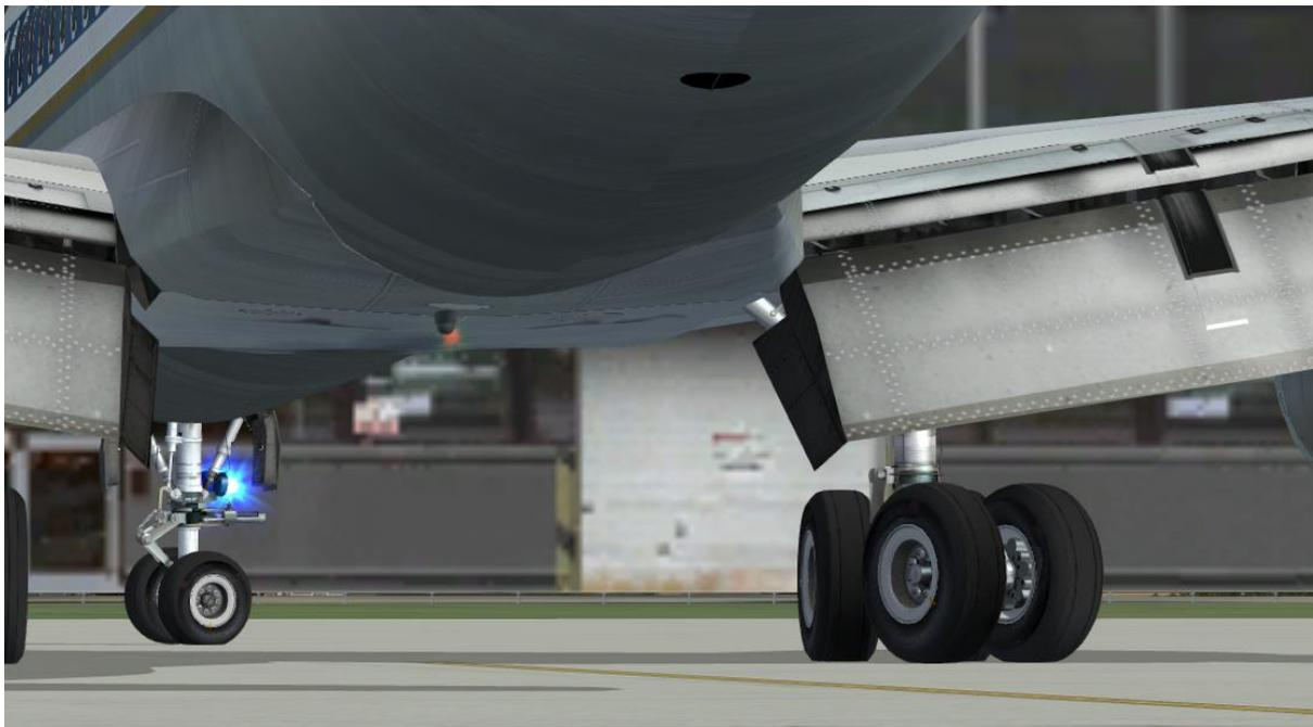
The bogies are also designed to remain level when the weight is lifted from the gear. They do not droop like they do on most modern aircraft, which allows for a more compact retraction system.
