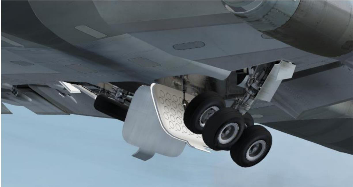
Towards the tail of the aircraft, under the fuselage, is mounted the pressure relief vent door for the cabin pressurisation and air conditioning system. Opening and closing this door is simulated by using the [Shift]+[E]+[4] keys or the relevant switch in the virtual cockpit.
