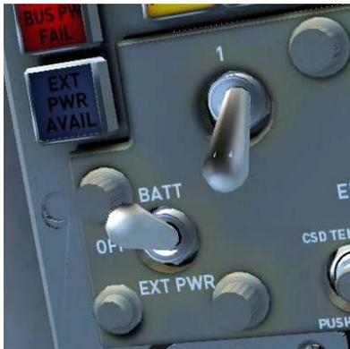
Rotate the VOLT & FREQ knob to the **BATT** position and verify that the battery is supplying voltage.
