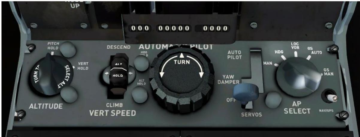
The aircraft is fitted with an independent autopilot and flight director. This means that you can select different modes on the flight director and autopilot at the same time, for example HDG mode on the autopilot and VOR LOC mode on the flight director.
