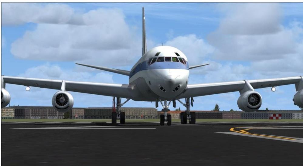
The engines fitted to the early DC-8s were turbojets which operated with reverse thrust capability and 'silencers' called ejectors which extended aft to cover the exhausts in an attempt to reduce noise. These ejectors carried the reverser buckets which, when reverse thrust was selected, closed completely over the exhausts and directed the gases forward.
