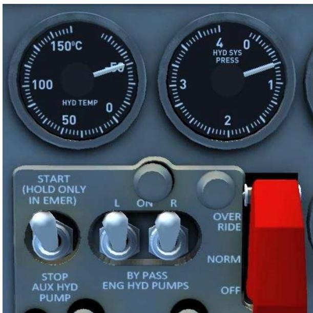
Switch off the auxiliary hydraulic pump before moving on to the engine management panel, checking that the engine oil quantity for each of the four engines is at its maximum value.
