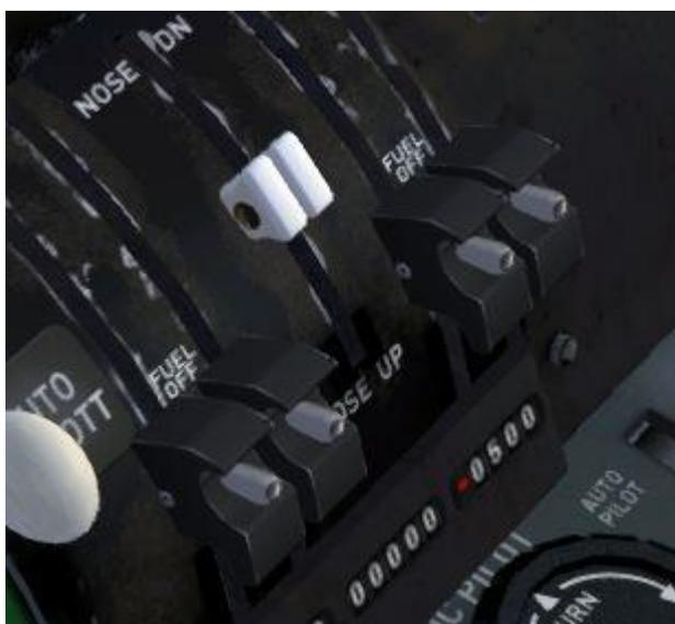
On the Engineer's panel, move the engine 1, 2, 3 and 4 tank levers to the **OFF** (down) position and switch **OFF** the boost pump switches.
