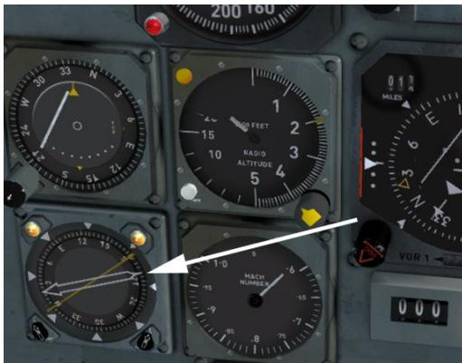
Once the aircraft has stabilised on a direct course towards the VOR, rotate the AP SELECT knob to select navigation hold mode (**LOC/VOR**). The aircraft will turn to intercept your GPS flight plan to Kansas City.
