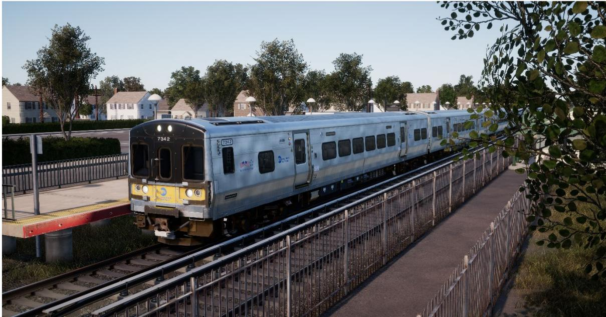
Electrification of the LIRR began in 1905 and today virtually all its west-end trackage and approximately half its total track miles are electrified with 750-volt DC power delivered via third rail. The present-day workhorse of the LIRR is a fleet of 836 M7-class EMUs constructed by Bombardier, the first of which entered LIRR service in 2002.
