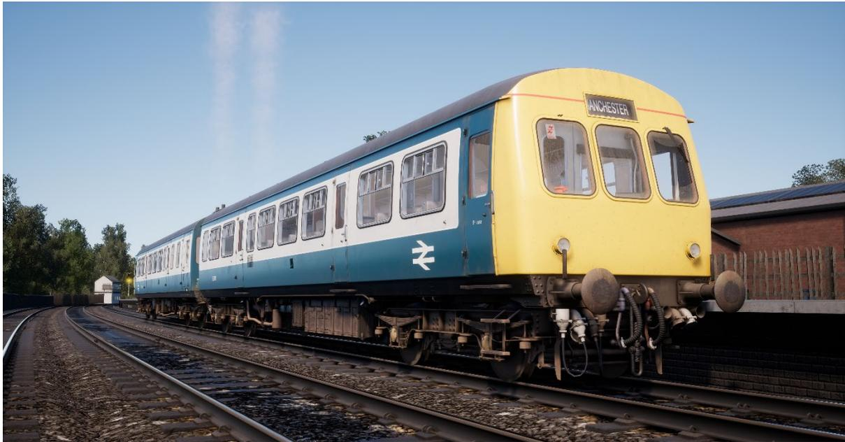
The Class 101 was one of the largest classes of first-generation Diesel Multiple Units on the British railway network. Built by Metro-Cammell Works in Birmingham from 1956, the Class 101 was made up from a number of sub-classes, making them the most numerous and possibly most successful and well known of first generation DMUs.
