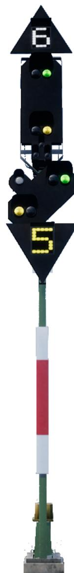
◀ This is a variation on the example signal. In this case, the distant works exactly the same except that the presence of the white light tells you that the next main signal is closer to the distant than normal so you will need to react more promptly.
