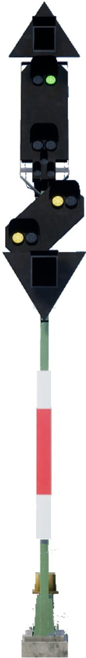
In this example we are approaching a signal which has an Expect Stop distant aspect. This tells us crucially that the next main signal is a Stop aspect and we must not proceed past it.
