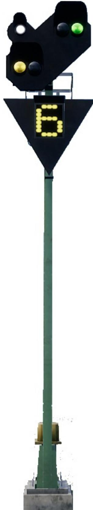
◀ This variation is slightly different again, note that there is no Ne2 white board. This, combined with the white light, means that this is a repeater and is used to provide additional sight of a following distant signal.
