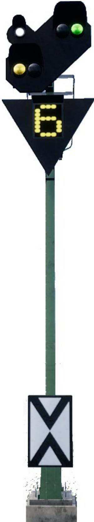
◀ In this variation, we have just a distant signal and it has a white light. The presence of the Ne2 white board means this is an actual distant and the white light tells us that the following main signal is closer than it would normally be.
