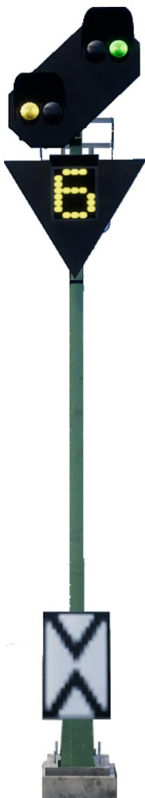
◀ This is a standard distant signal. Note the presence of the so-called “Ne2” board – a white board with two triangles touching, it looks almost like it has a cross. This signal is telling you about the state of the next main signal.
