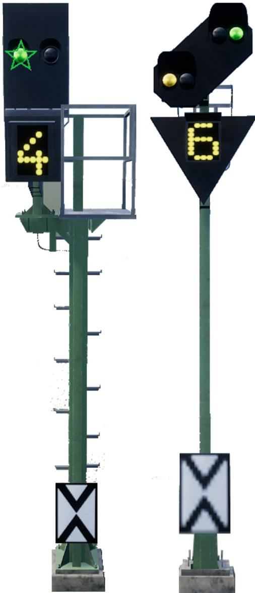
The signals below are also identical in the information provided. In this case, the white light combined with the Ne2 tells us that the main signal following this “Expect Stop” aspect is closer than normal, and we’ll need to brake accordingly.
