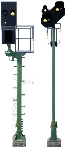
These signals are both distant repeaters (note the lack of Ne2 board), but also observe that the white light is now in the bottom left of the Ks signal.
