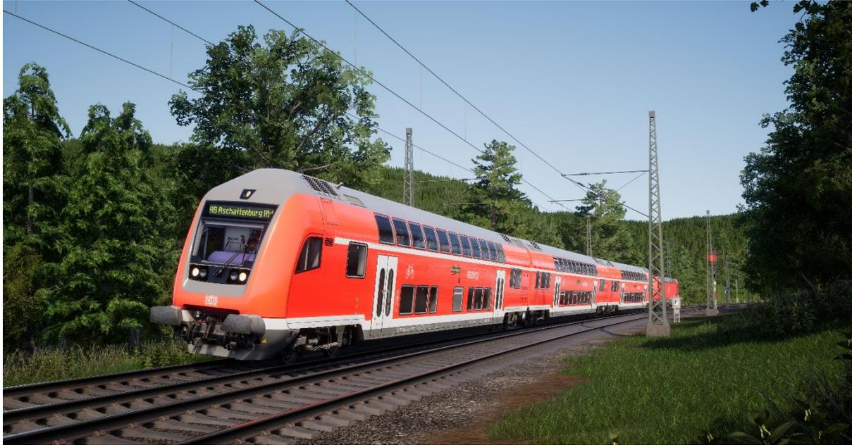
The DBpbzfa control car is an unusual driving position in that the driver is in the end of a passenger coach that has no actual capability to move on its own. Instead, this control car will remotely control the locomotive situated at the other end of the consist.
