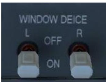
We keep the window heat on, to both avoid ice accretion and, interestingly, to keep the windows supple and more able to absorb the damage of a bird strike during the take-off phase.
