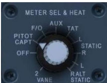
Out here on a beautiful clear day in the tropics, we have no need for either wing or engine anti-icing during the take-off but we will engage the pitot heat now to protect the pitot sensor.
