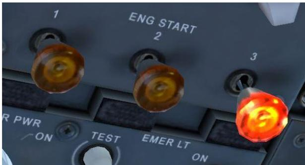
Below the ignition switch are three engine start switches. We can now start engine number 3 by pressing the third engine start button.
