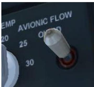
We can now also engage the avionics airflow, which provides cooling to the avionics equipment. This little switch can be found at the top right of the centre area of the panel, just to the right of the AFT CARGO TEMP rotary switch.
