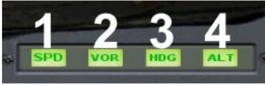
The Flight Guidance System Annunciator indicates which autopilot modes have been selected and engaged.
