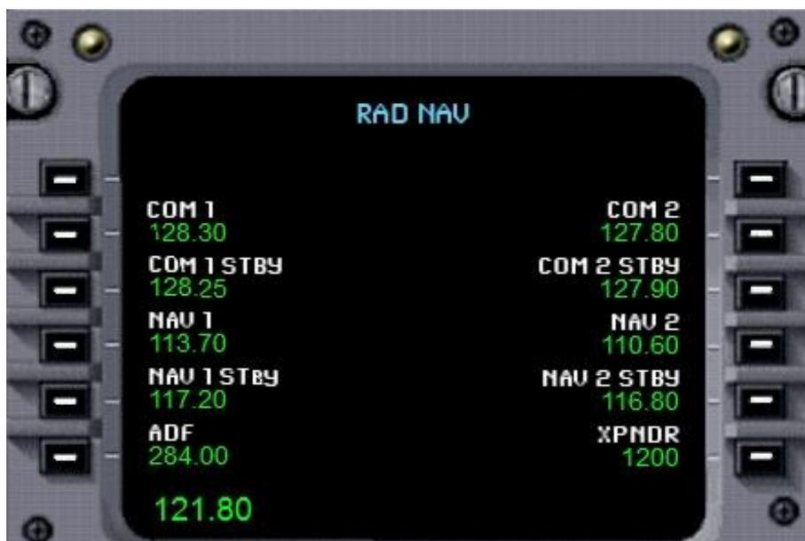
To input the value into Com 1 press the line select key 2L.
