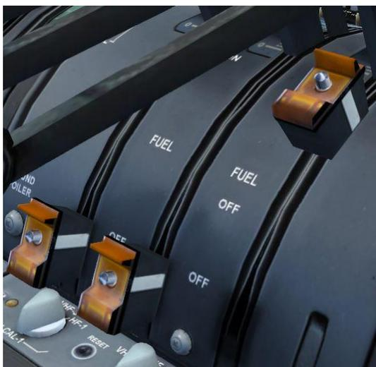
You will see immediate movement on the engine gauges on the panel. After two or three seconds supply fuel to engine number 3 for a full light-up by moving the fuel cut-off switch for the third engine (located on the pedestal) to RUN.
