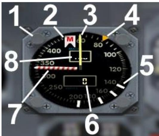
1. Knobs located in each corner of the gauge are used to control the position of the speed reference bugs
