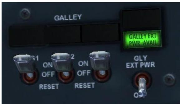
Finally, switch on the galley power using the three switches located at the top of the upper electrical panel.
