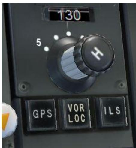
When we receive the “Resume own navigation” cue from ATC we can also transfer into an autopilot mode that allows us to track the flight plan in the FMC, in a manner identical to GPS NAV mode in a light aircraft. Press the GPS and then the VOR/LOC buttons in sequence. These buttons can be found under the heading window of the autopilot.
