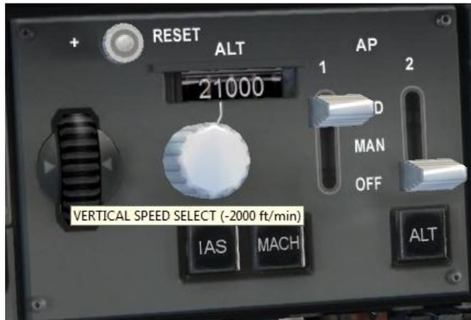
We will be descending in steps, following the guidance given to us by the controller. As each altitude is given, dial it into the altitude window, select a vertical speed of -2,000fpm, and press the ALT button to begin the descent. The procedure is exactly the same as the steps during climb, with the one exception of setting a descent of -2,000fpm using the thumbwheel rather than a positive climb.
