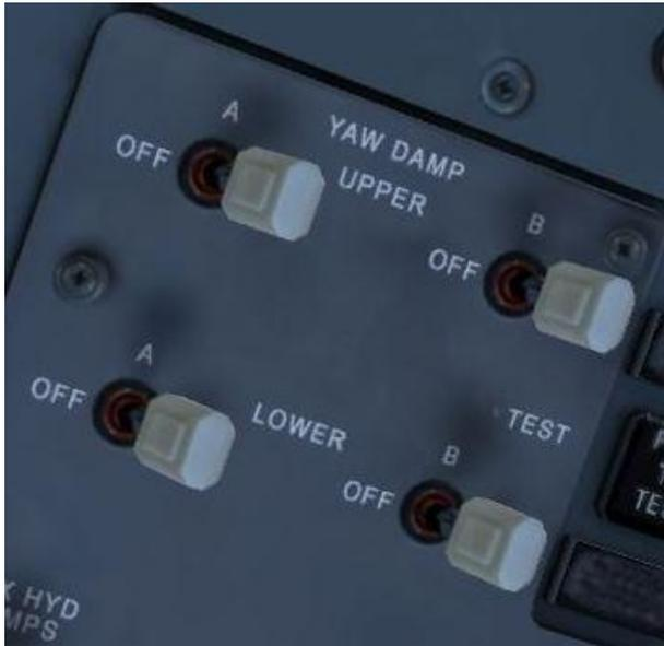
We can now return to the overhead panel to finalise our lights and instrument heating. Welcome back to those of you who skipped forward through the engine start procedure! We will also engage the yaw dampers; this stops the aircraft from 'dutch rolling', which is a particularly nauseating yawing motion that would more than do justice to any fairground ride you care to mention.
