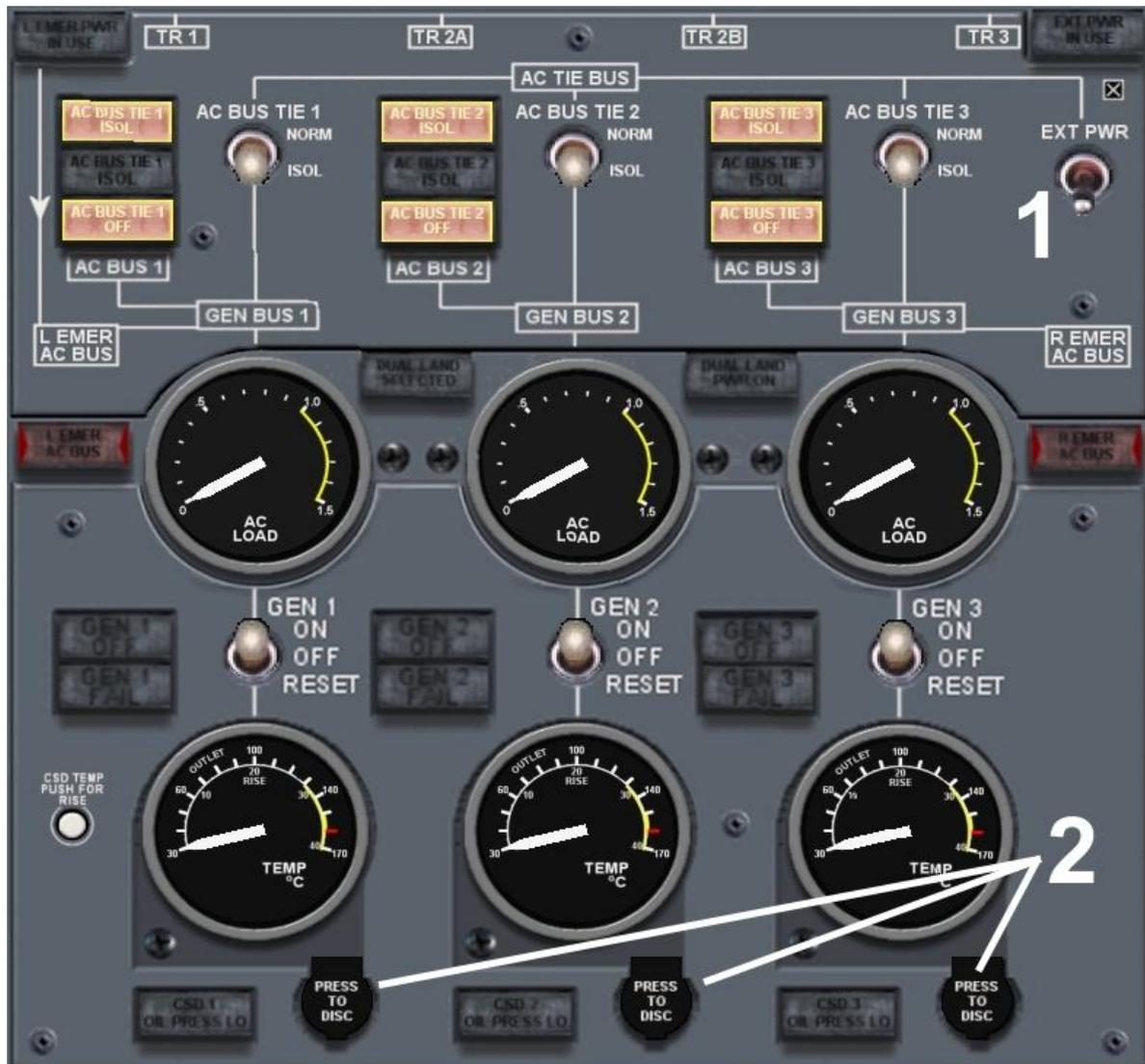
1. External power switch. With the aircraft parked and the parking brake set, this will supply electrical power to the aircraft.
