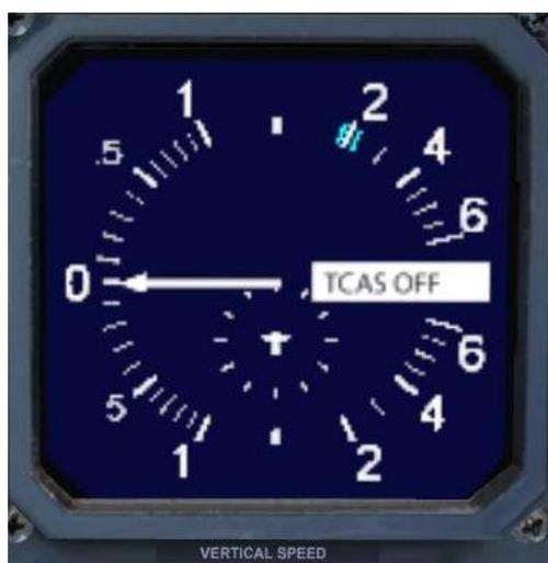
The actual vertical speed set is seen as a blue marker on the vertical speed indicator / TCAS panel on the centre left of the primary 2D panel under the primary altitude gauge. Adjust the thumbwheel until a vertical speed of 2,000 feet per minute is indicated on the VSI with the blue marker.
