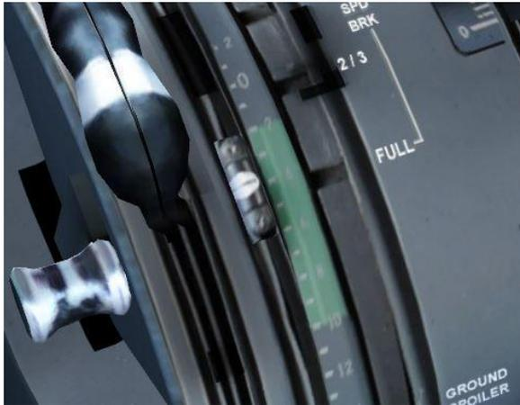
Open the pedestal and set the elevator trim to four units up.
