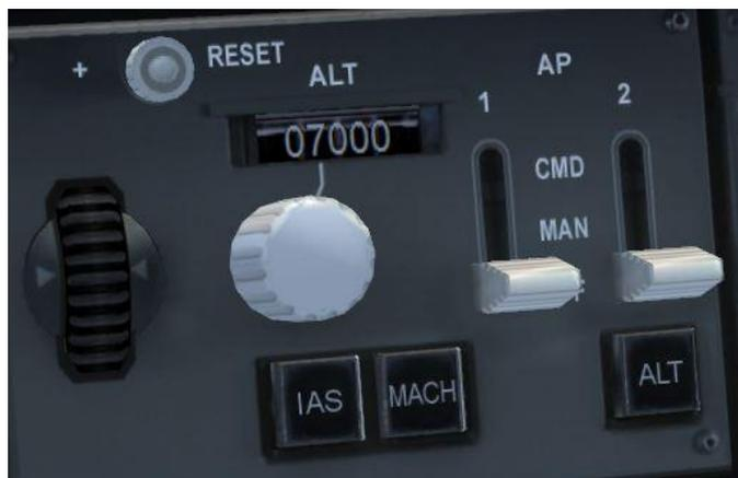
You will have been given an initial climb altitude, and we can enter this directly into the autopilot deck of the aircraft as we shall be flying using the auto-flight functions. The altitude window is the rightmost window on the autopilot panel, marked as ALT, at the top right of the glareshield. Dial in the altitude requested by ATC using the mouse over the rotary knob immediately below the window.
