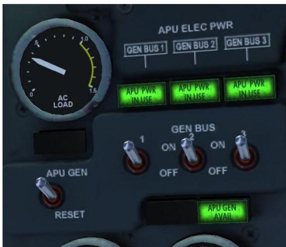
Now that the APU is running we can connect the APU to the electrical bus.
