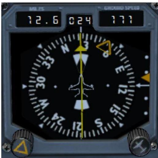
As the glideslope indicator starts to move down on the HSI, slow the aircraft to 160kt and deploy 22 degrees of flaps. As the glideslope centres and is captured by the autopilot, lower the gear, deploy full flaps and slow the speed by winding the speed window to our landing speed of 145kt.
