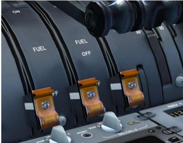
Open the pedestal panel and locate the small orange fuel cut-off switches below the thrust lever for each engine. Before we start the engines we need to ensure that these cut-off switches are set to OFF (the down position towards the bottom of the screen). Do this now with a simple mouse-click on each.
