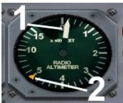
1. Radar altimeter indicator needle – indicated height AGL (Above Ground Level) from 1,500 feet and less
