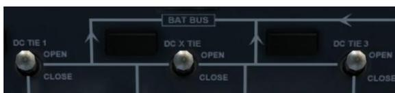
We can also go ahead and prepare the engine generators ahead of engine start by selecting the three DC tie switches at the bottom of the panel to the open position.
