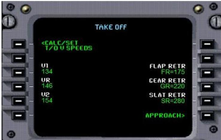
Open the FMC and press the button marked TOFF/APR (Take-off/Approach). At the top left of this page is an option to automatically calculate our take-off speeds, saving us a lot of time and effort! Press the button to the left of this prompt, and our take-off speeds will automatically be shown on this page as V1, Vr, and V2
