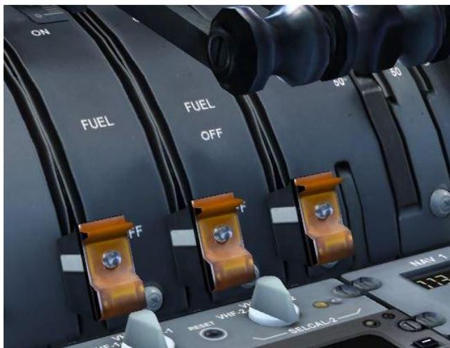
The ATC controller will give us guidance to the gate. On arrival at the gate allow the APU to power the electrical systems using the technique described previously and apply the parking brakes. Switch off all three engines by putting all three engine cut-off switches on the pedestal to the OFF position.
