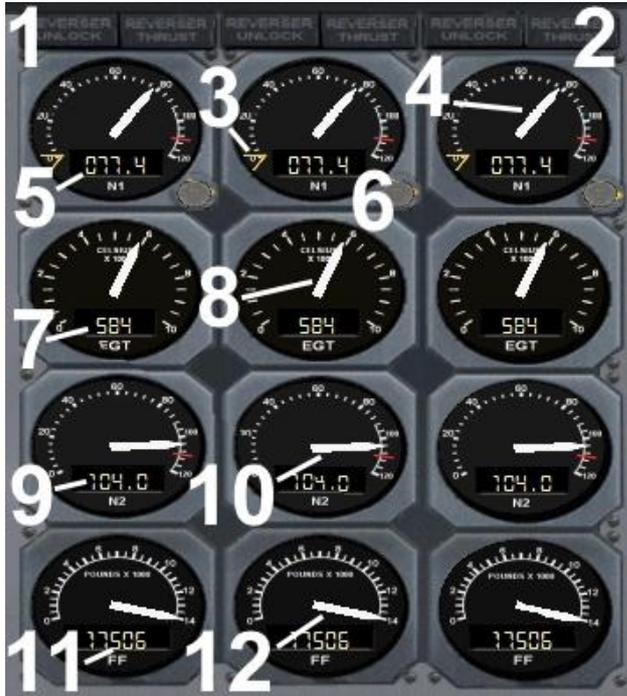
1. The REVERSE UNLOCK caption illuminates to indicate the unlocking of the corresponding engine thrust reverser.
