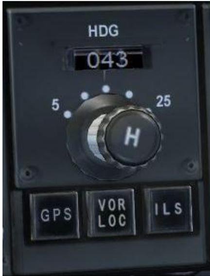
As you take the centreline of the runway, come to a stop and hold the aircraft steady with the brakes. We can now align the autopilot heading window with our current runway heading, so dial in the heading of the centreline now, as ATC has asked us to maintain runway heading after departure.
