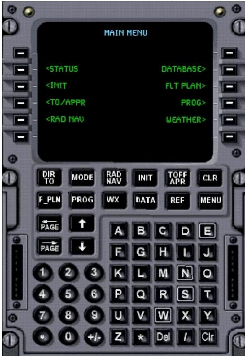
The FMC (Flight Management Computer) in this F-Lite aircraft utilises the internal flight planner in Flight Simulator and so there is no lengthy procedure needed to input a flight plan into the FMC.
