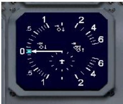
Traffic is displayed on the Vertical Speed Indicator. The switch to turn on the TCAS is located on the transponder unit mounted in the pedestal. Traffic is indicated by different colour-coded images.
