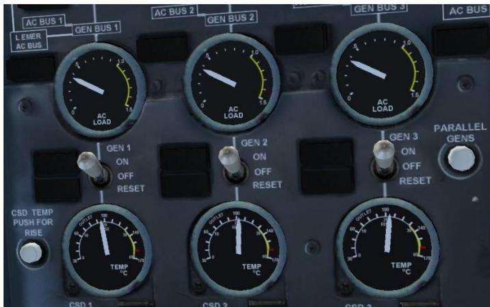
Open the engineer's panel and connect the engine generators to the electrical system. They can be found at the very bottom left of the engineer's panel.
