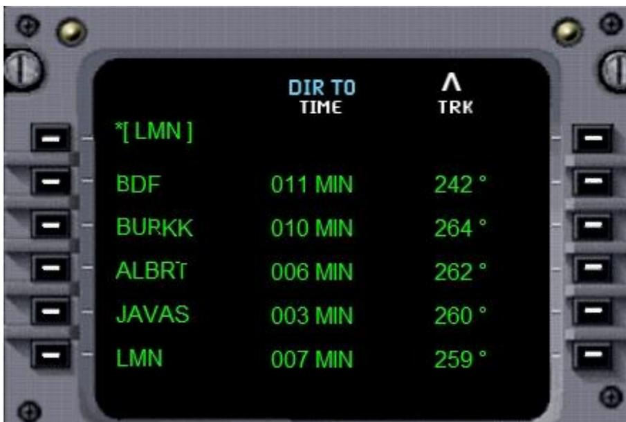
Now press the line select key 1L to finish the command. Your flight plan will now fly directly to LMN, skipping over the other waypoints. This is done using the GPS feature on the autopilot.
