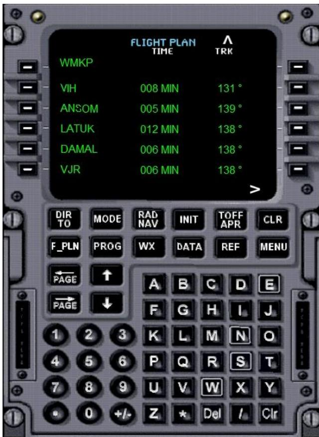
We can now return to the main panel and confirm that our flight plan is indeed in the flight management computer (FMC).
