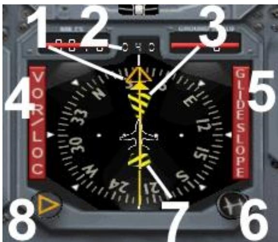
1. Heading bug – set via the AP or the heading bug knob on the HSI
