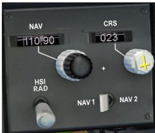
As we start our descent we can tune the ILS for our arrival runway. We will be landing on runway 2L, to the north, flying a wide sweeping arc over the island on our final approach. So let's go ahead and set up the radio frequency for the ILS. Using the NAV1 receiver at the top of the glareshield, enter the frequency of 110.9 and a course of 023, which is our inbound course to the runway.
