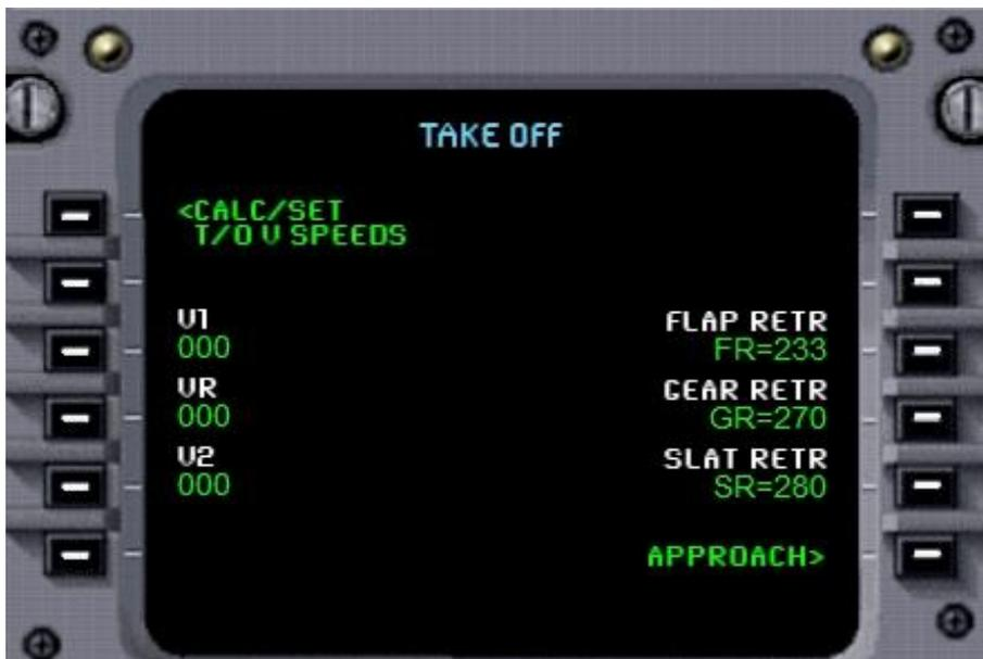
Pressing the line select key 1L will calculate your V-speeds using your current weight and air density:
