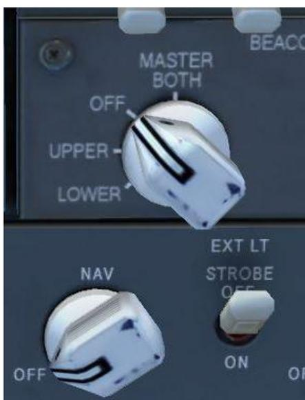
Once the engines have spooled down, switch off the navigation and beacon lights with the controls on the overhead panel.
