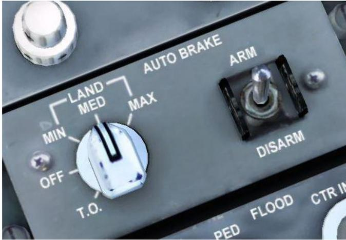
As we cross the centreline of the runway the aircraft will automatically capture the localiser and turn us inbound on our final approach. We can now arm the autobrakes and spoilers for landing. Both switches can be found on the lower left of the pedestal panel.
