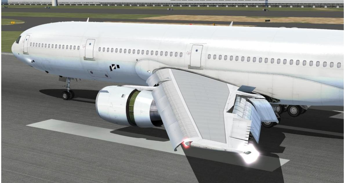
Once clear of the runway, retract the flaps, lower the spoilers and configure the exterior lights. Start the APU, using the procedure described at the start of this tutorial, in preparation for gate arrival.
