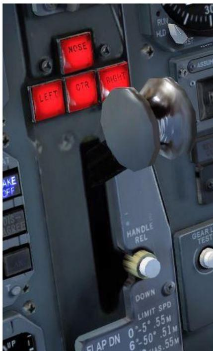
As we achieve a positive climb, raise the gear and also engage the autothrottle into speed tracking mode.
