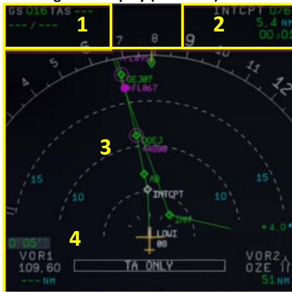
Picture 8: ND – Navigation Display (Standard)
