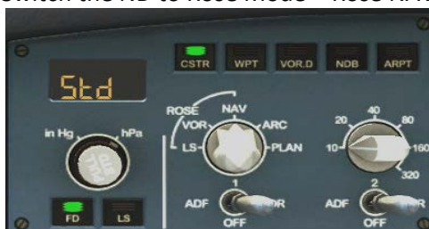
Picture 118: Settings for ND mode and range
