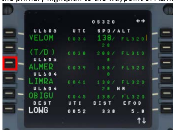
Picture 138: Enabling ALTN DEST – step 1
