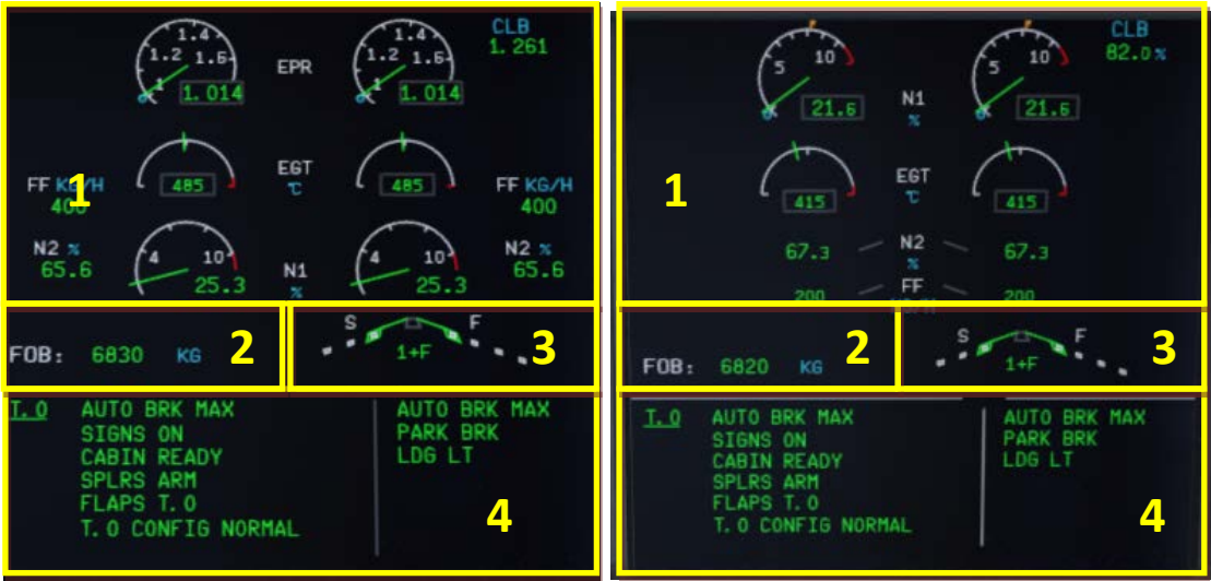
Picture 17: E/WD–Engine Warning Display with IAE resp. plane with CFM Engines
