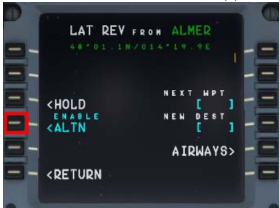
Picture 139: Enabling ALTN DEST – step 2
