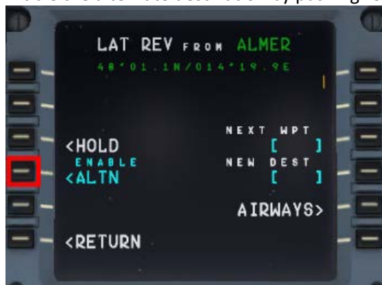
Picture 129: Enabling ALTN DEST – step 2
