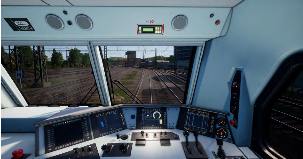
▲ The FT95 Unit Location in the DB BR 146.2, and the DB BR 766.2 DBpbzfa Control Car ▼
