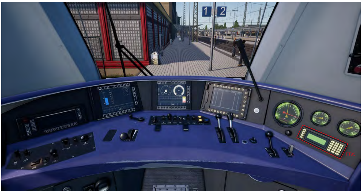
▲ The FT95 Unit Location in the DB BR 146.2, and the DB BR 766.2 DBpbzfa Control Car ▼
