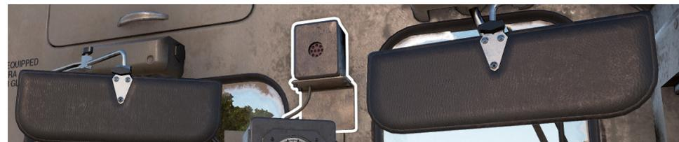
When the alerter is enabled, if you are travelling at over 5mph it will begin a countdown from 65 seconds (there is no visual representation for this). Once that countdown reaches zero it will make a sound in the cab and turn an indicator on. On the HUD, you will also see the Alerter icon light up.
