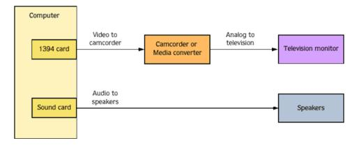
The video is converted to DV format and sent through the IEEE-1394 card to the DV device (camcorder or DV-to-analog media converter). The DV device sends analog output to the television monitor.
