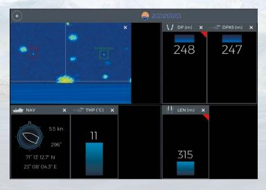
Here you can customize the sensors display which is shown on the primary screen when sitting at the trawler control deck. If you press the + button at the top left you can drag different measurement panels from the menu which will appear. Most measurements will only have valid data when you are actively trawling.
