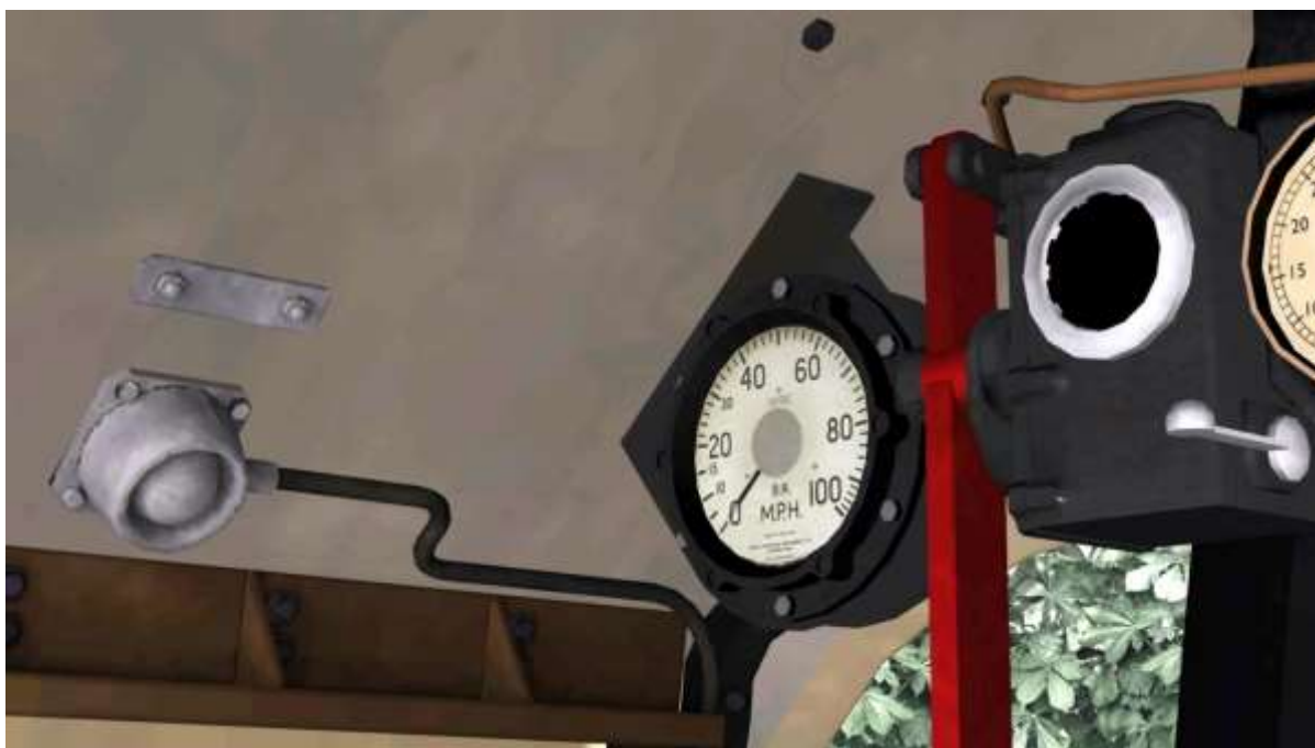
Example of a cab equipped with AWS and speedometer
