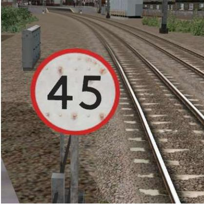
These signs display the permissible speed in M.P.H. applicable to the section of line beyond the sign up to the commencement of any subsequent permissible speed section.
