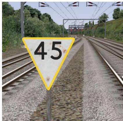
These signs provide advance warning of a reduction in permissible speed ahead. Permanent AWS Ramps (Automatic Warning System) are often installed in conjunction with these signs. In these cases the driver must cancel the AWS warning when triggered on approach to these signs.
