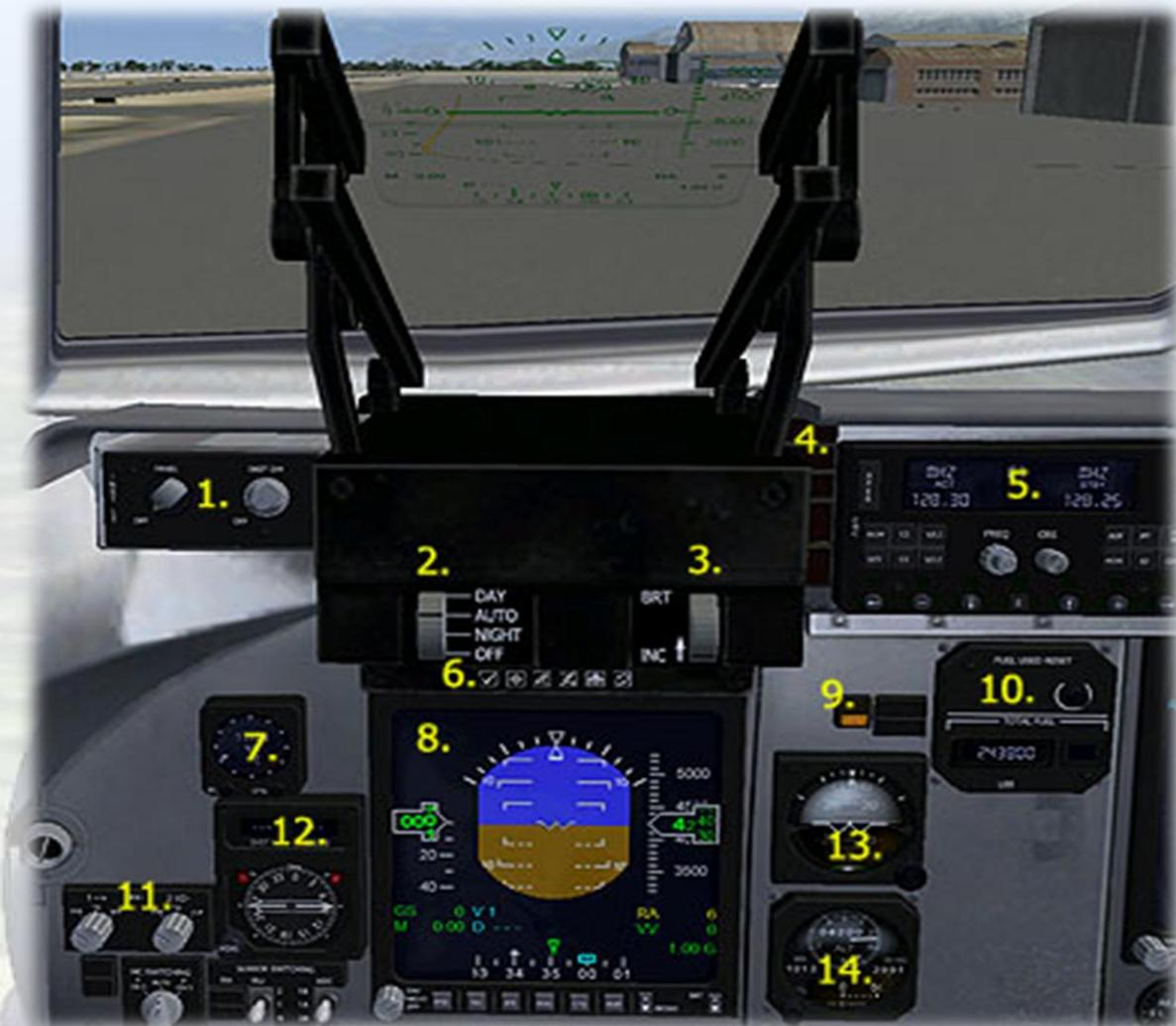
1) Cockpit lighting. Left knob toggles cabin lights, right knob has three position dimming of all digits (not MFDs), use right-click to return to full brightness.
