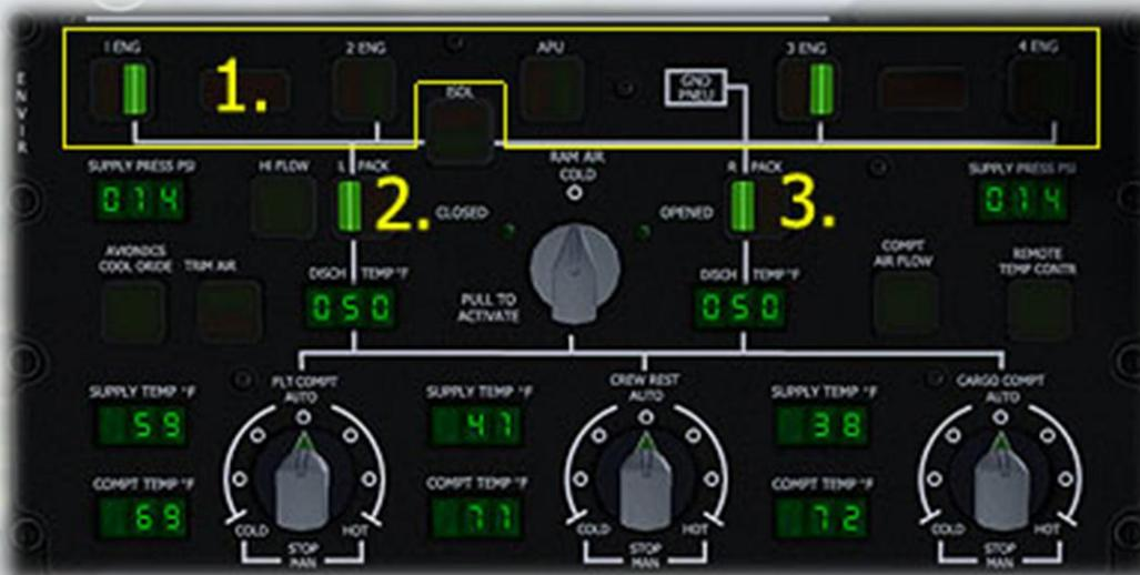
1 - Engine/APU Bleed Air Switches. At least one bleed air switch must be on in order for the left or right air conditioning packs to work. If no engines are running, the APU can be started and bleed air from that used to power the packs.
