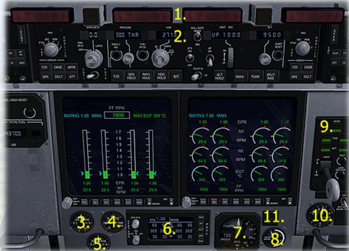
1) Fire Extinguisher Handles. These 4 (one for each engine) T-bar handles will both shut down the engine and extinguish the fire when activated. Use the mouse RIGHT click to activate them. A fire can be set in the FSX Failures section to test their operation. NOTE: fires can not be set in FS2004.
