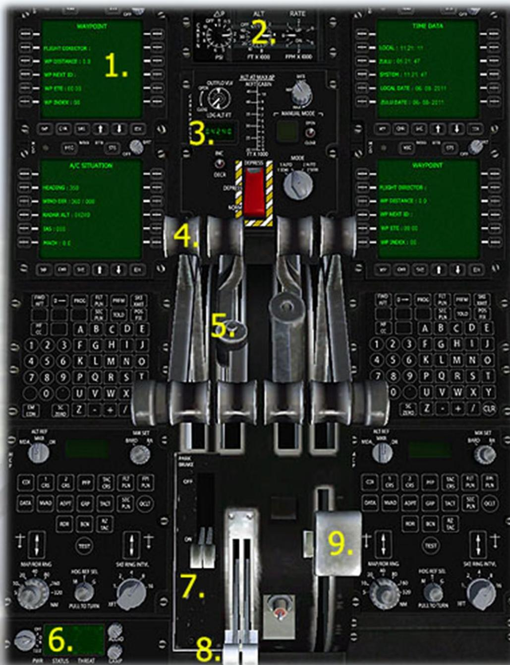
1) Mission Computer Display (MCD) (4, simulated). The MCD's are non-functional, although each can be independently switched on or off and on each, the lower two left buttons can be used to display waypoint, aircraft situation and time data. It is hoped that a suitable Flight Management Computer can be integrated into the model at some point in the future.
