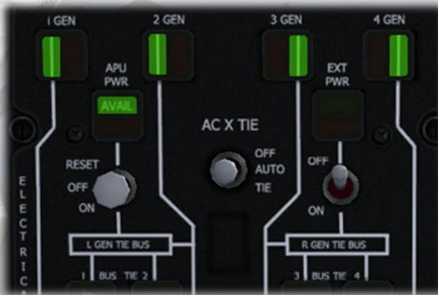
5) Electrical Panel. The four generators can be switched on or off here. The 'APU PWR' lamp indicates that the APU is on and power can be used from its own generator if required.
