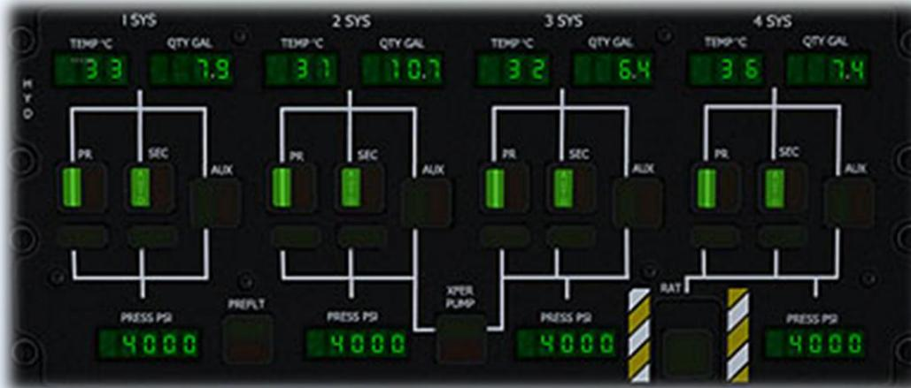
4) HYD Panel. This area of the overhead is not interactive, it merely displays the status of the four hydraulic pump systems. On starting a particular engine, the Auxiliary pump lamp will come on to prime the Primary and Secondary pumps. Once the pressure in the system has reached 4,000 PSI, the Auxiliary pump stops and the Primary and Secondary pumps take over. The digital readouts along the top display the temperature and quantity remaining of the hydraulic fluid in the four systems.
