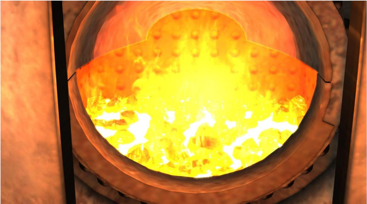
In the above picture, the fire is at the ideal fire mass, the coals should just cover the row of stay heads. As the fire mass drops the stay heads become much more visible and below around 360lb fire mass the firebars can begin to be seen.
