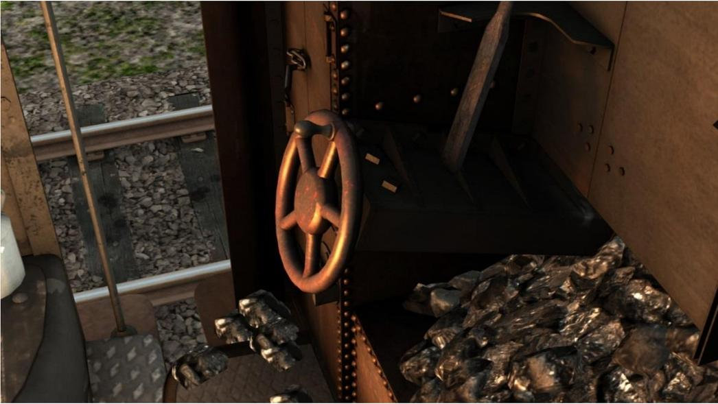
The hand brake is used to manually apply the brakes on the tender, it can be used to assist in gradually buffering up an unfitted train. However, it is not a very powerful brake and so the vacuum brake will need to be used to assist in stopping long trains. It can be applied using the ‘/’ key and released with ‘**Shift** + /’.
