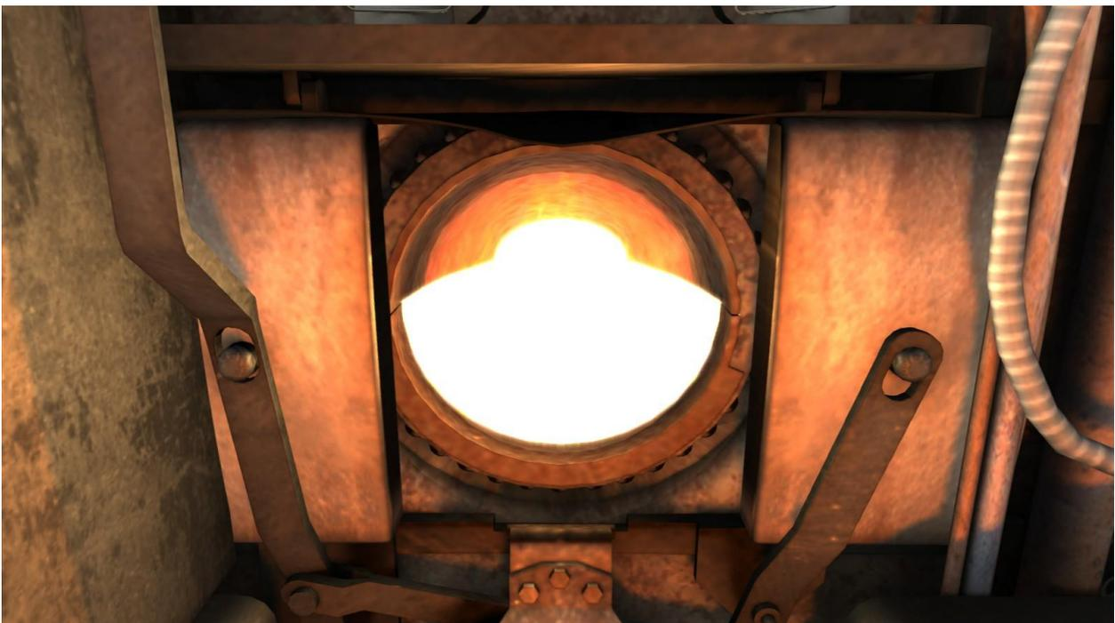
Figure 4. Both the fire and the firebox are incandescent white and it is practically impossible to distinguish where the fire bed is.
