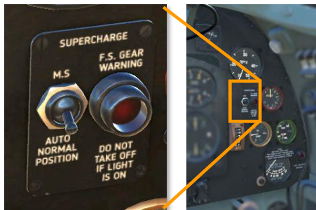
Figure 71: Supercharger control panel
