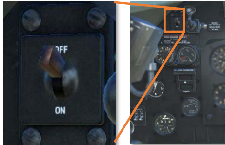
Figure 60: Navigation light control switch
