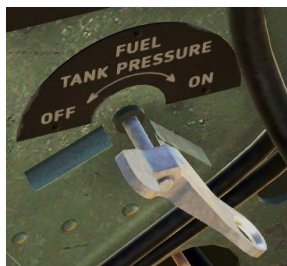
Figure 84: Fuel tank pressure valve
