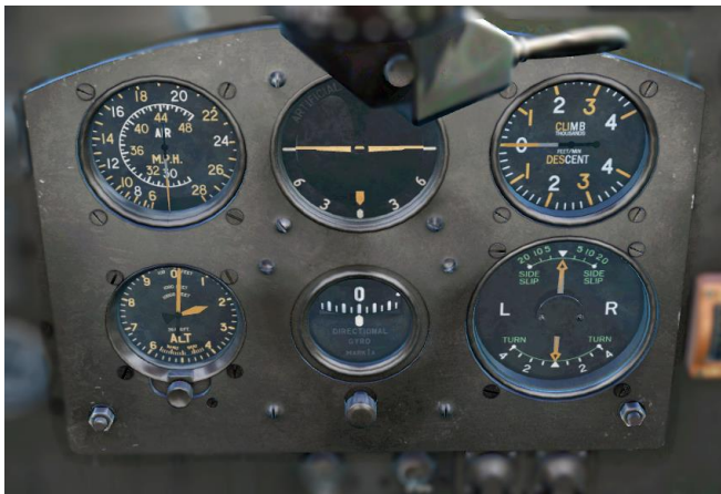
Figure 50,: Blind-flying panel (late model)
