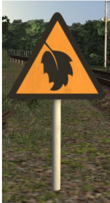
Poor adhesion area starts
