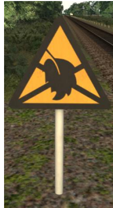
Poor adhesion area ends
