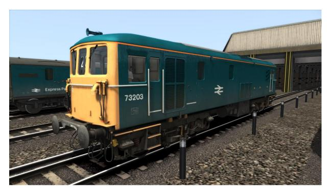
The Class 73 is an electro-diesel locomotive designed as part of the British Railways 1955 Modernisation Plan.
