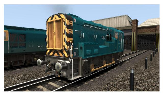
The British Rail Class 09 is a class of 0-6-0 diesel locomotive designed primarily for shunting and also short distance freight trips along branch lines.
