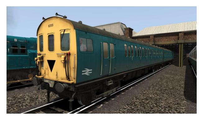
British Rail Class 416 (2 EPB) electric multiple units were built between 1953 and 1956. They were intended for inner suburban passenger services on London's Southern Electric network. There were two subclasses of Class 416: Class 416/1 to an SR design on salvaged 2 NOL underframes, and Class 416/2 to BR's Mark I coach design.
