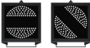
A banner repeater signal indicates whether the signal ahead is displaying a proceed aspect or is at danger. Modern fibre optic banner repeating signals, as shown opposite, consist of a rectangular unlit black background displaying a white circle with a black bar.
