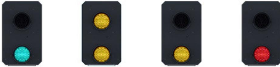
Colour light signals are used for controlling running movements. They display aspects by means of red, yellow and green coloured lights.
