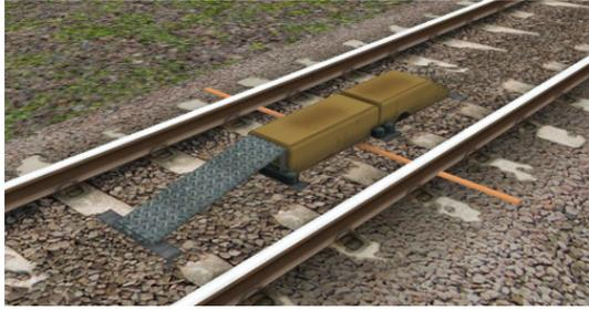
AWS is provided to give train drivers in-cab warnings of the approach to signals, reductions in permissible speed and temporary/emergency speed restrictions, and to apply the brakes in the event that a driver does not acknowledge cautionary warnings given by the system.
