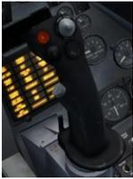
The side stick was one of the major innovations of the F-16. It was located to the side of the cockpit so the full arm of the pilot could be supported making high G manoeuvres easier to control. Furthermore the stick was almost fully static. It did not move as other controls in aircraft did. It senses force applied to it and not movement. We added a tiny bit of animation to give the user some feedback though. There are no controls on the side stick for the FSX pilot.
