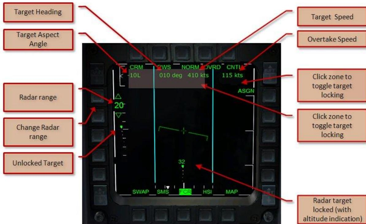
One of the more complex bits of information on this screen is the Aspect Angle. It has nothing to do with the position of the target in relation to your heading but only shows the angle between the (extended) tail of the
