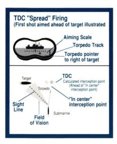
**The TDC:** American submarines had an analog "Torpedo Data Computer" (TDC) that calculated a torpedo's correct course. The crew had to input the target's course, speed and range.
