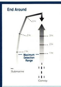
Initially the submarine spots a northbound convoy. To make an "end around", the sub turns parallel to the convoy and moves northward on the surface.
