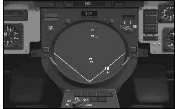
The Moderate/Authentic Mode TID showing targets displayed in Range-While-Search Mode.
