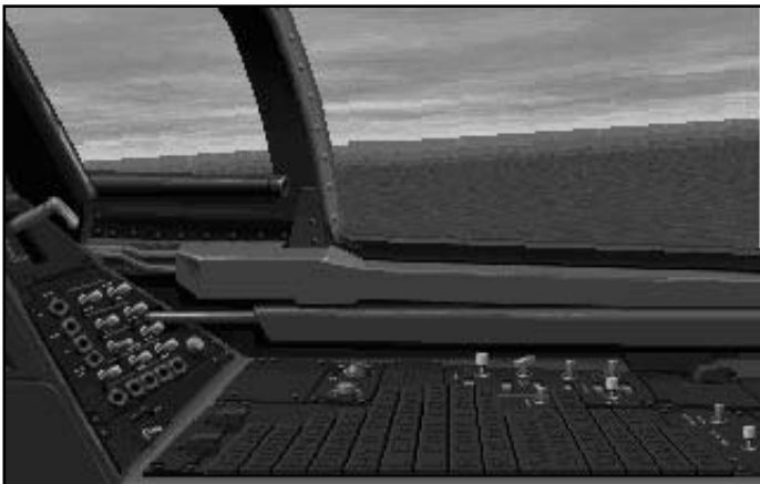
The Pilot's right hand console. In foreground is the column of lights known as Master Caution-Advisory panel. When these lights are On, you know you've got problems.
