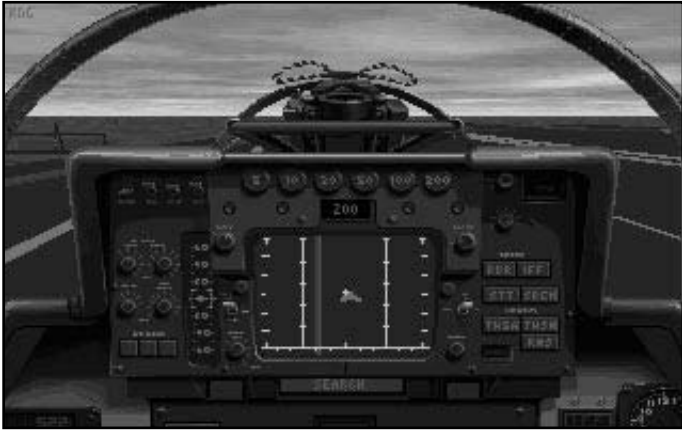
The Standard Mode Detailed Data Display (DDD) in SEARCH mode displays targets like a conventional radar screen.
