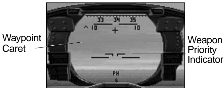
The basic Head-Up Display (HUD) showing pitch ladder and Phoenix missiles in priority.
