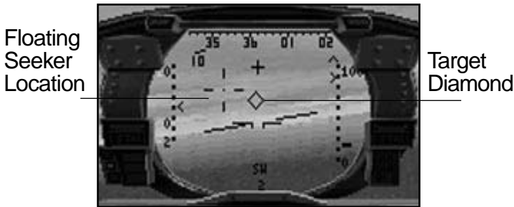
The Head-Up Display (HUD) with the floating AIM-9 Sidewinder seeker-head looking for a target.
