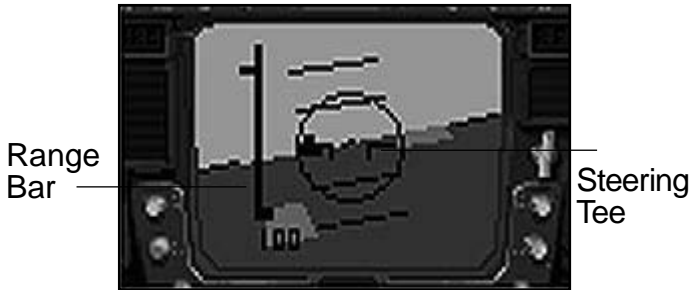
The Vertical Display Indicator (VDI) in combat mode showing a locked target and target range bar.
