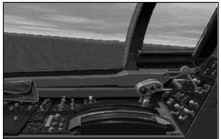
The Pilot's left hand console. The throttle is the prominent feature on this particular view.
