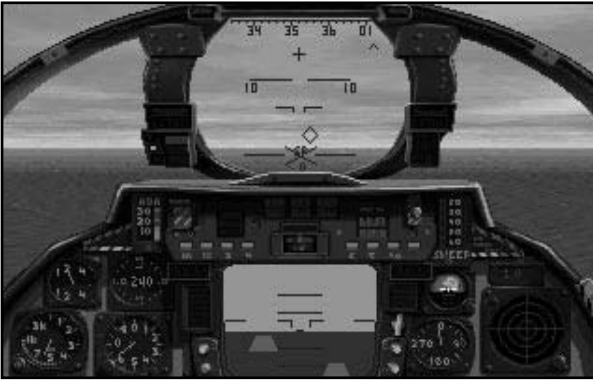
The Moderate/Authentic Mode HUD showing the Vertical Scan Lock-on (VSL) diamond.
