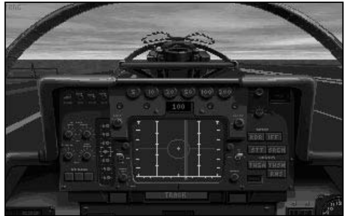
The Standard Mode Detailed Data Display (DDD) tracks single targets by focusing the radar beam. Note that you lose sight of the other targets while you are in TRACK mode.
