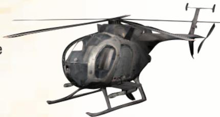
**LITTLE BIRD:** This highly maneuverable helicopter is designed for light attack and close air support. It can be configured with benches for troop transportation, with machine guns, or rockets.
