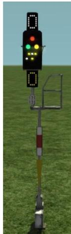
**Combined Signal Type: Hp/Ks Vr Zs3 Zs3v**
