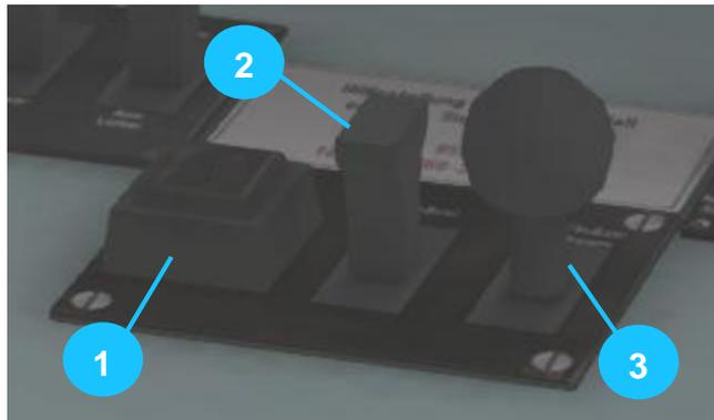
PZB controls on the Cab Desk of a BR101 (other locomotive controls would be similar but not identical)
