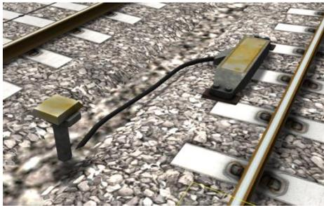
The PZB system incorporates in-cab signalling. This is where the control desk has indicators, alarms and buttons that will react according to the signalling status on the railway. The mechanism by which this works is a series of “balise” magnets placed on the side of the track. An example of one of these magnets is shown in the image on the left.
