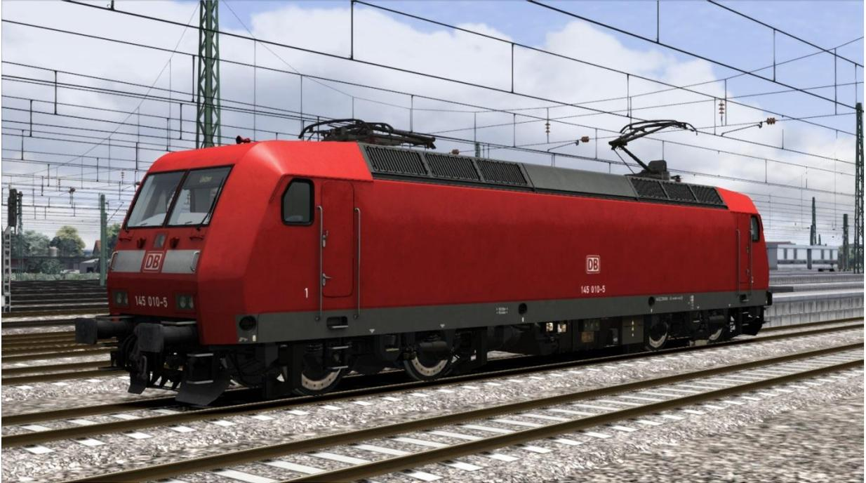
The DB BR145 is a Bo'Bo' mainline electric locomotive built by Adtranz primarily for the Deutsche Bahn at the end of the 1990s. The BR145 is primarily a freight locomotive but was also used for passenger operations.
