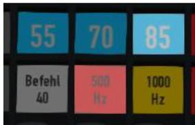
As we pass the 500hz magnet, we must have slowed down to 65km/h (40m/h) or else we might not be able to stop in time for the signal. If that's the case, the PZB system will apply the emergency brakes. There is no need to acknowledge the 500hz magnet. At this point, the 500hz light on the control desk will activate, indicating the current restriction.
