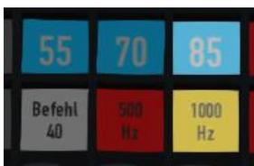
Note that there is no alert in the cab when we pass over the 1000hz magnet. This is because the driver is expected to be aware that they have passed a Distant Signal and react accordingly. Once the PZB Wachsam/ Acknowledge control is pressed, the display will update to indicate that the locomotive is now in a monitored state. As we are a Type O train, the 85 light and the 1000hz light will be activated.
