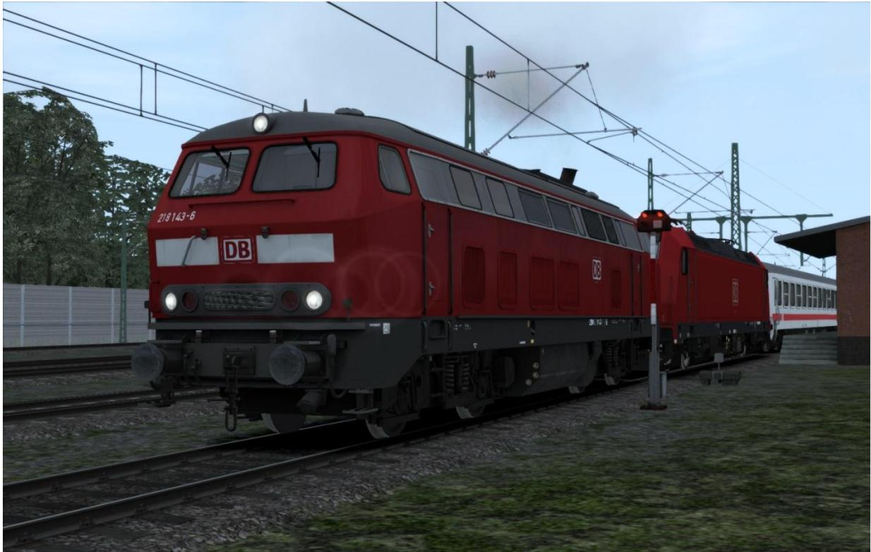
The DB BR218 (before 1968 the DB BR V 164) are a class of 4 axle, diesel hydraulic locomotives acquired by the Deutsche Bundesbahn for use on main and secondary lines for both passenger and freight trains.
