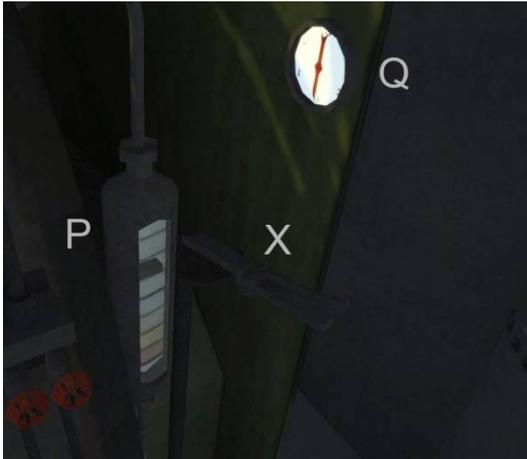
The control labelled **X** is the oil regulator. As the oil burner has a very small fire mass the regulator will need almost constant adjustment when working up a grade so it is recommended you use the built in auto fireman. The absence of a significant fire mass means that the fireman must attempt to adjust the firing rate to meet steam usage rates. Since the burn rate is controlled by the exhaust rate, if the exhaust steam gets too high, the fire mass will drop and even go out.
