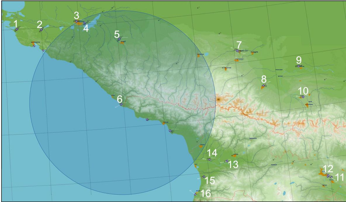
**Image 9.8:** RSBN/PRMG ground stations at various airports, with channel numbers (1 – 16). RSBN ground station range/coverage is given for Sochi-Adler only (showing range/coverage for all RSBN's would cover entire image). [This image is available for hi-resolution print \(Mods\aircraft\MiG-21BIS\Doc\Manual\\_Images\).](#)
