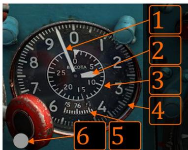
The Barometric altimeter (VDI-30K) measures barometric altitude up to 30km. The small needle (2) points to an altitude in km (scale 3) while the big needle points tens of m (1). The pilot can set the desired atmospheric pressure in window (5) using button (6).
