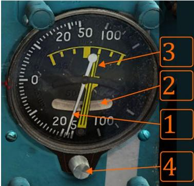
The DA-200, often referred to as the “variometer”, will give you precise information about vertical velocity up to 20 m/s, and rough information from 20 m/s to 200 m/s. The Slip ball (2) will indicate slip, while the turn indicator (3) will show you the turn rate. This indicator is specially designed to indicate bank up to 45° in steps of 15° when the airplane is flying at 500 km/h IAS. The purpose of this function is to replace the KPP if it fails, and enable safe landing pattern creation.
