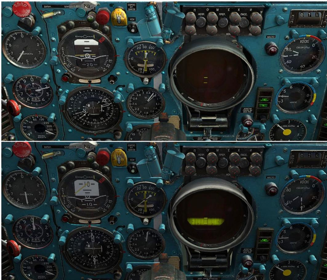
**Image 9.12:** Upper image shows aircraft at 71km from RSBN station, while in CLOUD PENETRATION mode. Note the glide path is below aircraft (glide needles) while vertical speed is within recommended by glide director needle (yellow needle on KPP). On the lower image the same aircraft is 24km away from RSBN station, on glide path and currently descending with greater than recommended vertical speed.
