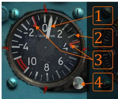
The Accelerometer shows current (1) and maximum/minimum g-load (3) achieved during flight. Maximum and minimum loads can be reset using button (4). This is a very important instrument, especially if the aircraft has external loads and g-load needs to be controlled to avoid the load falling off, possibly damaging the airframe or other planes in formation, or causing damage to civilian infrastructure or people.
