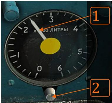
The Fuel quantity indicator shows overall remaining fuel state in liters. Knob (2) serves to set initial fuel quantity (pre-flight setup). If the fuel delivery system fails, e.g. fuel from wing tanks is not being used for some reason, indicated fuel quantity will be higher than the actual amount available. Therefore,
