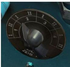
**Image 9.2: ARC frequency range selector** or sector selector (RV37). There are four sectors (1 - 4) and each sector has two sub-sectors (I and II). This allows the storage of 72 stations ( $4 * 2 * 9$ ).
