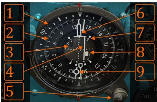
The Course System (NPP) is a complex instrument showing current magnetic heading, direction to a selected NDB or RSBN station (9, pointer at tail), desired course or radial (6, pointer at head, set up with button 5), correct reception of localizer (3, K - “kurs”) and glide slope (8, G - “glisada”) signals, aircraft position in reference to localizer and glide slope signals (central white needles), relative angles necessary for landing pattern creation (7) and relative
