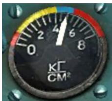
The Engine oil pressure gauge displays the current engine oil pressure. Normal engine oil pressure is 3-4kp/cm<sup>2</sup>. The Engine low oil pressure warning light (CM54) will illuminate if the engine oil pressure drops below 1kp/cm<sup>2</sup> or metal particles are detected in the engine oil. Detection of metal particles indicates severe engine problems which can lead to total engine failure.
