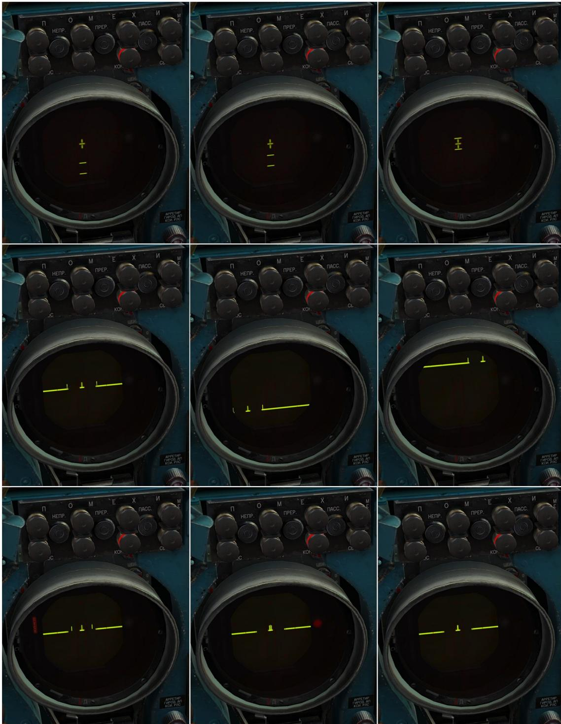
**Image 10.7:** illustration of radar self-test pattern
