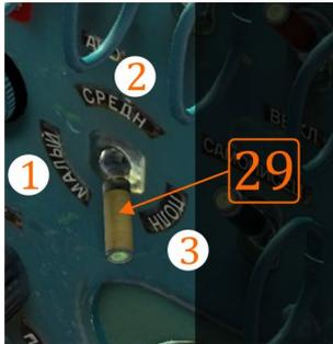
External lights are positional lights and landing/taxi lights. Control switch for positional (AKA formation) lights is located on the right vertical panel (RV29). This switch has four positions: neutral position - lights OFF, position 1 - small intensity lights, position 2 - medium intensity lights, position 3 - maximum intensity lights.
