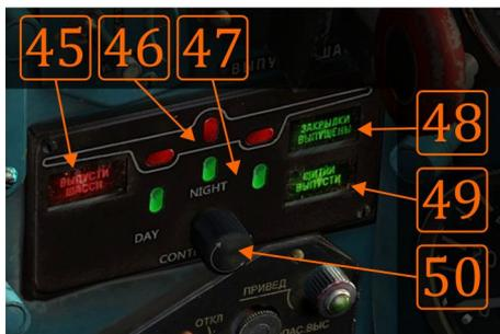
PPS indicates the state of the landing gear, flaps and air brakes. Warning light (LV45) indicates that flaps are extended while the landing gear is retracted; the message reads “*Extract landing gears*”. Light (LV48) indicates that flaps are extended. Light (LV49) indicates that air brakes are fully extended.
