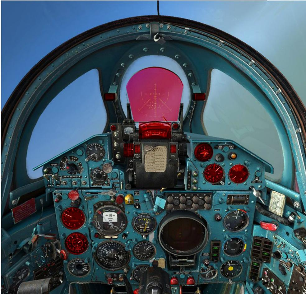
**Image 8.8:** Instruments you should check often during the combat maneuvering. Look outside the cockpit most of the time.
