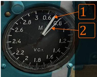
Thick needle (1) shows the M number starting from 0,6 M. Thin needle (2) shows the TAS starting from 600 km/h (on 0,6 mark). Scale indication follows this logic.
