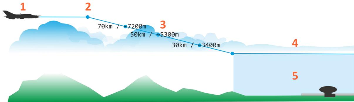
**Image 9.9:** Guidance program for CLOUD PENETRATION mode
