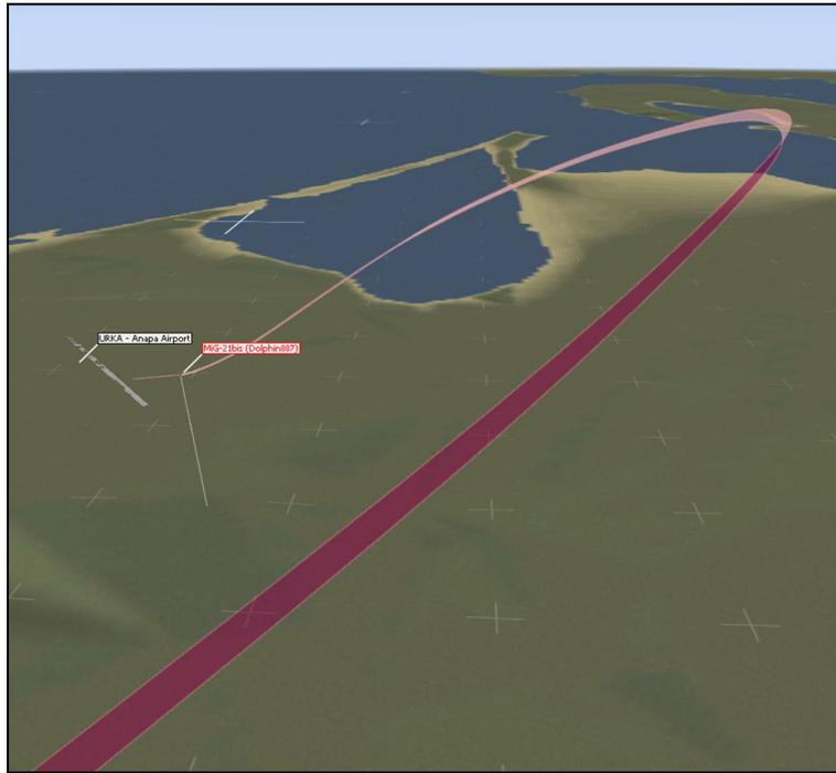
**Image 8.5:** Semi-turn over could be a bit tricky to visualize if you've never seen it. The image shows an aircraft turn-diving to the left, changing its heading by  $\sim 90^\circ$  during the maneuver. This maneuver is often used for ground target attack, since the MiG-21 has poor down-forward visibility. Thus the target should be off to the side prior to the attack run.
