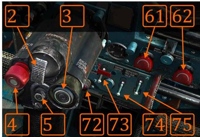
**Image 10.13:** Tactical release switch (CL73) and BOMBS ARMED light (CL72). CL61 and CL62 are payload jettison buttons under the red caps.
