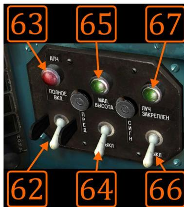
**Image 10.6:** Main radar control panel.
