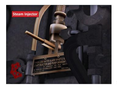
The Steam Injector is a precision piece of equipment which uses a venturi system to use high pressure steam to push water from the tender into the boiler under pressure through a check valve which only allows water into the boiler if the pressure behind the water exceeds the pressure in the boiler.
