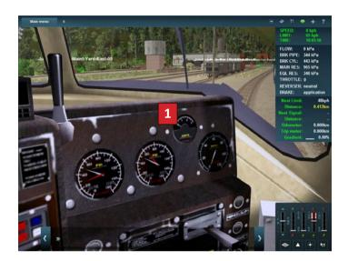
The Load Indicating Meter or Ammeter provides the best guide for throttle handling when accelerating a train. By observing this meter, it will be noted that the pointer moves to the right (increased amperage) as the throttle is advanced. Thus for maximum acceleration without slipping, the throttle should be advanced one notch each time the pointer begins moving back toward the left, until full power is reached in notch 8.
