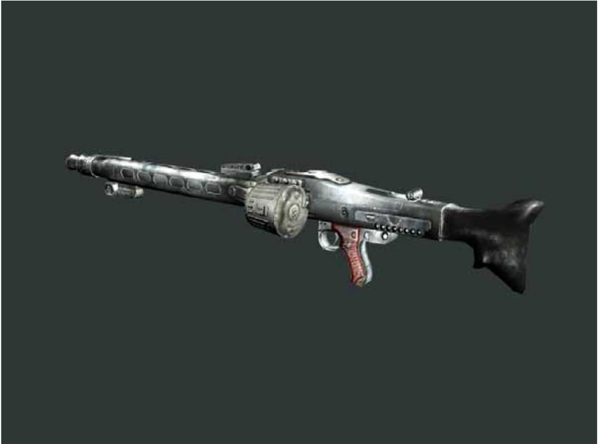
**MG-42 Medium machine gun.** This gun has the percussion mechanism fixed at the breechblock. The launching mechanism enables only automatic fire. Besides, it has high rate of fire – up to 2400 shots a minute, though such rate can shake the gun. To enable accurate shooting it is recommended to make short series of 5-7 shots. Due to its light weight (6.5 kg.) it can be used both as a stationary weapon and a hand held gun
