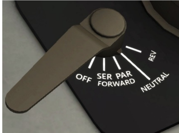
Reverser showing Neutral, Reverse and the two Forward settings; Series and Parallel.
