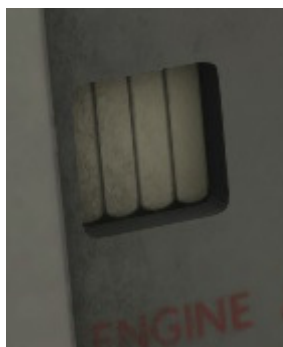
Status of diesel engine from left to right. Off, running up / down and on.
