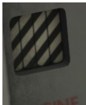
Status of diesel engine from left to right. Off, running up / down and on.
