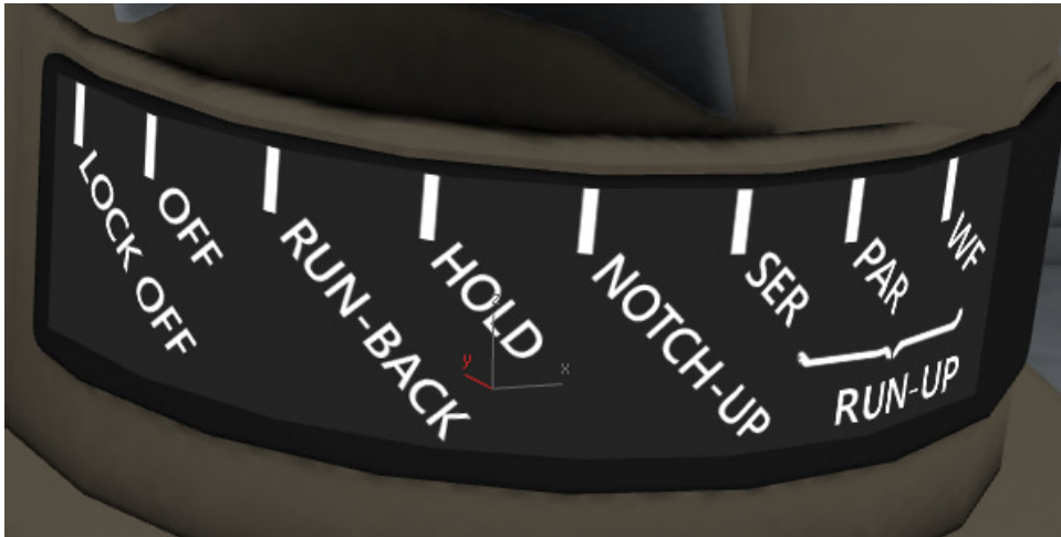
Electric Throttle Handle showing all power settings.
