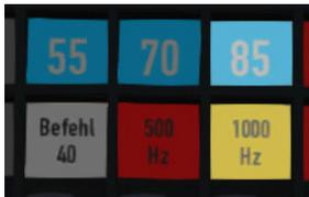
Note that there is no alert in the cab that we have passed over the 1000hz magnet, the driver is expected to be aware that they have passed a distant signal and react accordingly. Once the PZB Wachsam / Acknowledge control is pressed the display will update to indicate that the locomotive is now in a monitored state. As we are a Type O train, the 85 lamp is lit and the 1000hz lamp lights up.
