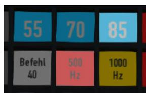
As we pass the 500hz magnet we must have slowed down to 65km/h or else we might not be able to stop in time for the signal and the emergency brakes will be applied. There is no need to acknowledge the 500hz magnet. At this point, the PZB lamps on the control desk will change to light up the 500hz lamp, indicating the restriction we're now in.
