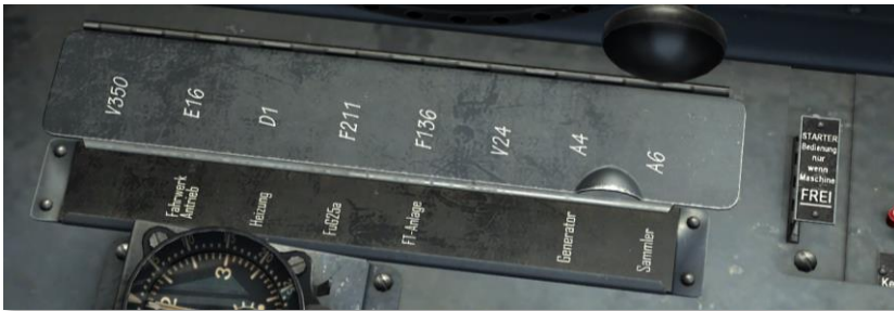
Figure 84: Circuit breaker cover down
