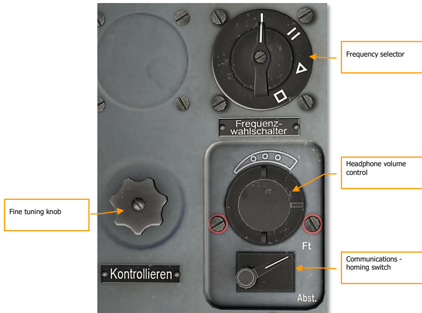
Figure 81: FuG 16ZY controls
