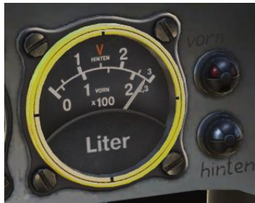
Figure 66: Fuel contents gauge with fuel warning lights
