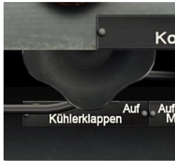
Figure 57: Manual radiator flap control
