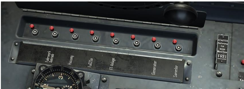
Figure 85: Circuit breaker cover up
