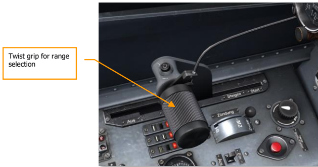
Figure 44: Throttle lever with twist grip and cable
