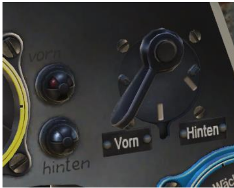
Figure 24: Fuel warning lights (left) and fuel gauge selector switch (right)
