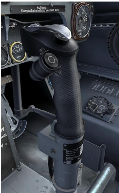
Figure 36: Flight stick, trigger, and bomb release button
