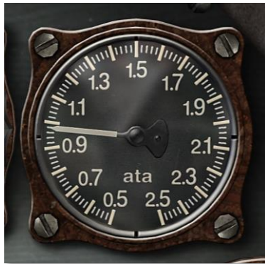
Figure 54: Supercharger pressure gauge
