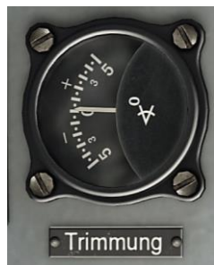
Figure 79: Horizontal stabilizer trim indicator
