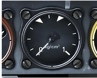
Figure 18: Water/Methanol pressure gauge
