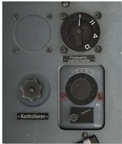
Figure 33: FuG 16ZY frequency selector, receiver fine tuning control, and volume control
