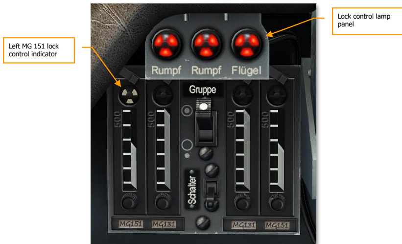
Figure 48: SZKK 4 with ammo indicators
