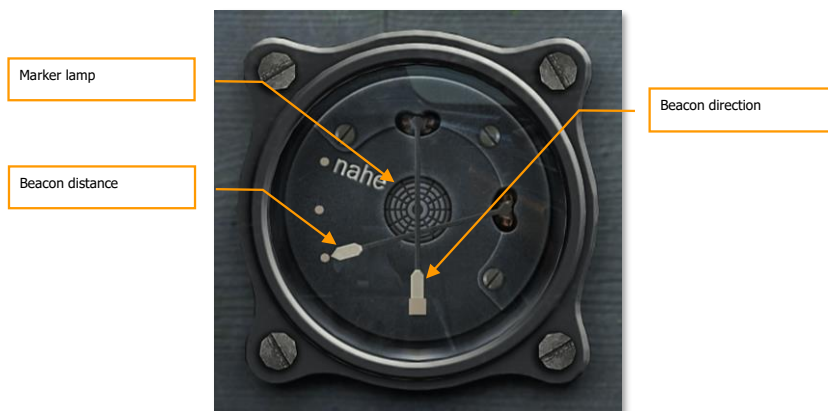
Figure 49: AFN-2 homing indicator
