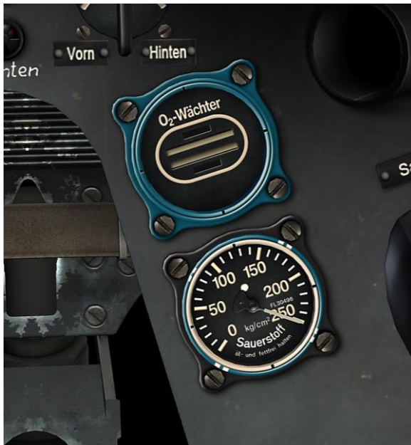
Figure 30: Oxygen flow indicator and pressure gauge
