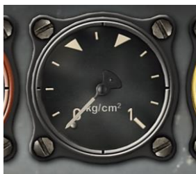
Figure 65: Water/Methanol pressure gauge
