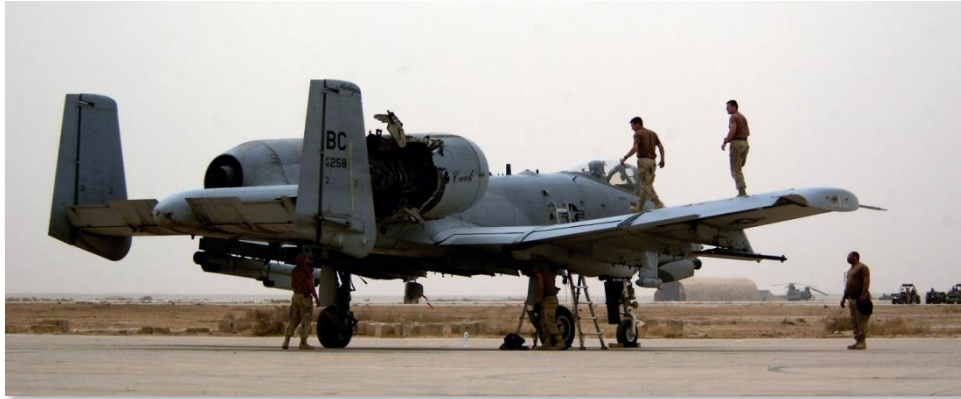
Figure 28. A-10 Thunderbolt II maintenance members inspect aircraft after it was hit by an Iraqi missile
