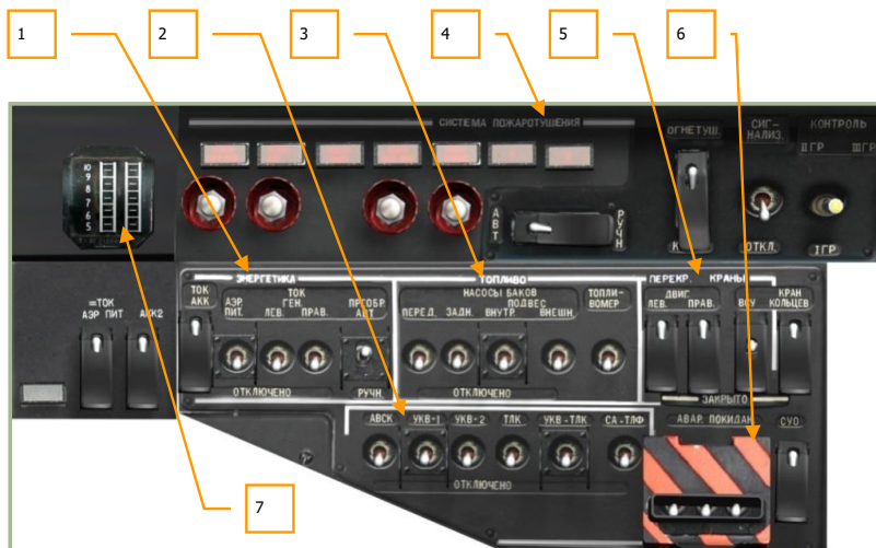
6-50: Wall panel, forward section
