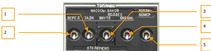
6-54: Fuel pump controls
