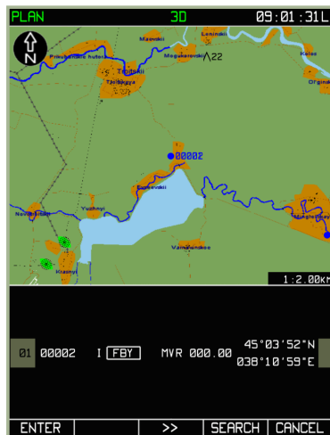
7-35: MENU/PLAN sub-mode display after successfully completing a navigational point search by use of callsign
