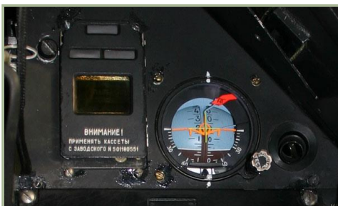
1-5: Ekran built-in warning and control system (left) and auxiliary flight indicator (right) in Ka-50 cockpit
