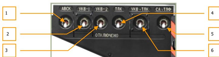
6-53: Radio and data link power control panel
