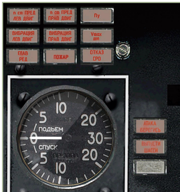
6-28: Caution light panel
