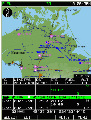
7-71: Loaded route before inverting
