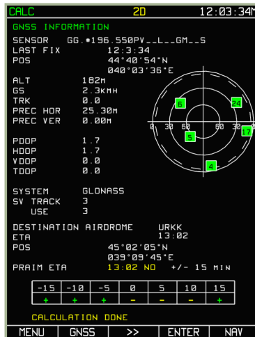
7-104: Automatic preparation of data for viewing of the almanac and making RAIM prediction calculations for the airfield of destination
