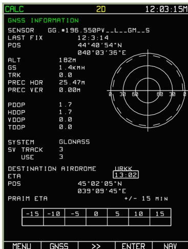
7-104: Automatic preparation of data for viewing of the almanac and making RAIM prediction calculations for the airfield of destination
