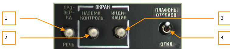
6-67: EKRAN Warning System and ALMAZ Voice Message Unit ("Betty") BIT controls
