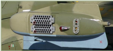
1-8: UV-26 flares dispenser, left (red) navigation light and the signal flare cartridge dispenser
