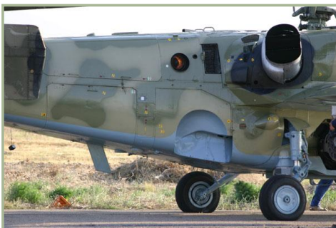
1-3: The exhaust nozzle of auxiliary power unit (in operate) and screen-type exhaust devices of main engine
