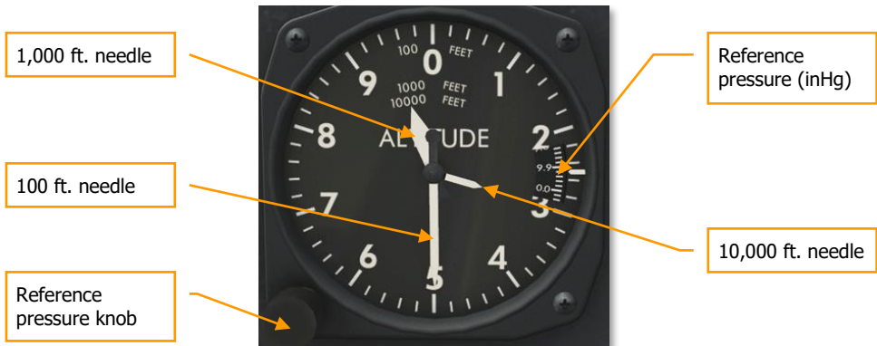
Figure 45: AN5760-2 Pressure Altimeter indicating 29,500 ft.
