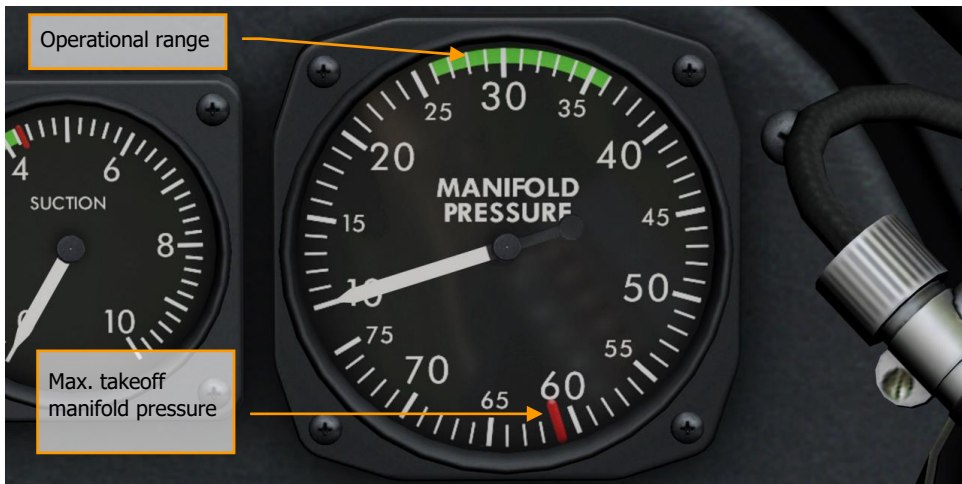
Figure 83: Max. takeoff manifold pressure – 61 in. HG (155 cm HG) (red mark). Operating range 26...36 in. HG (66.04 - 91.44 cm HG) (green zone).
