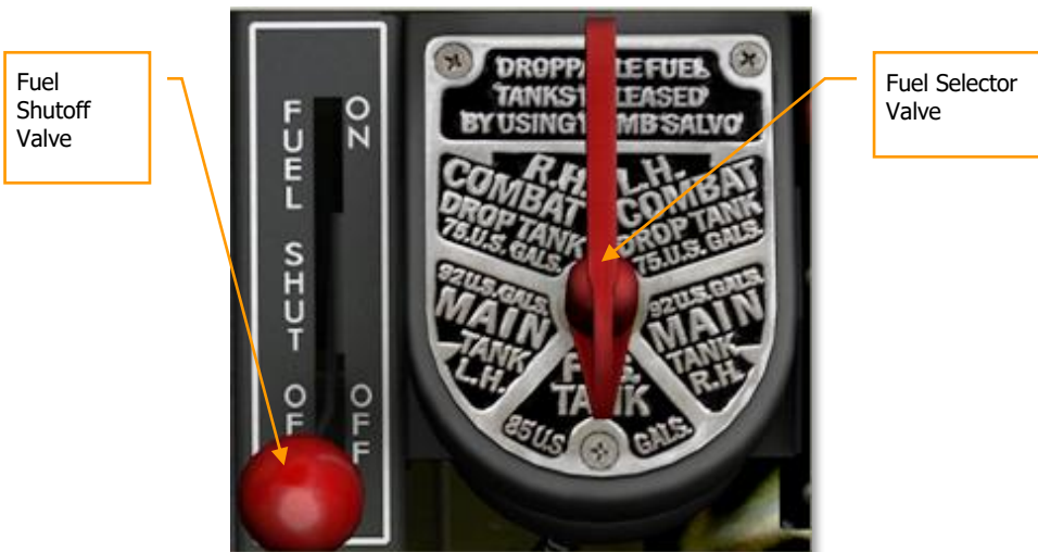
Figure 61: Fuel Shutoff and Selector Valves
