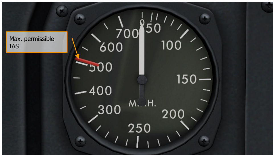
Figure 86: Max. permissible IAS 505 mph (808 km/h, 440 knots)
