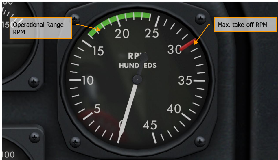
Figure 85: Max. take-off RPM 3000. Operating Range 1600...2400.
