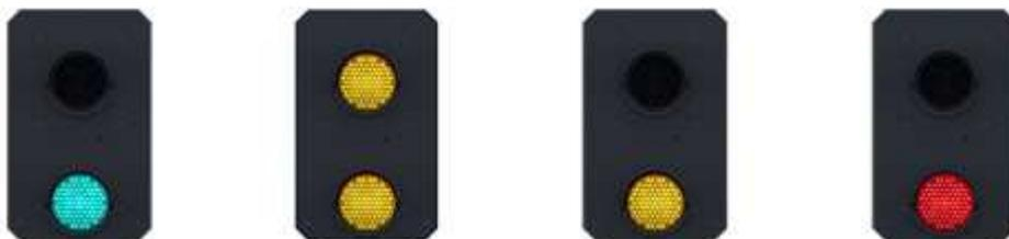
Colour light signals are used for controlling running movements. They display aspects by means of red, yellow and green coloured lights.
