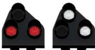
Ground Signals and Position Light Signals (PLS) display their aspects by means of the position and colour of lights. Ground Signals are always illuminated and can have miniature theatre indicators attached whereas PLS only illuminate to allow a train to pass in to an occupied section of line and are mounted as an addition to a main signal head.
