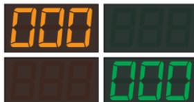
The yellow triple-zero is displayed to warn of an upcoming stop signal with an approach speed of 10 km/h. It's followed by the green triple-zero when the reduction is enforced.
