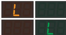
The yellow L is displayed to warn of a temporary speed reduction. It's followed by the green L when the reduction is enforced.
