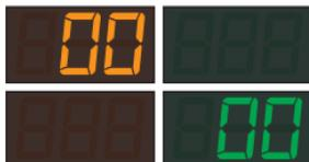
The yellow double-zero is displayed to warn of an upcoming stop signal with an approach speed of 30 km/h. It's followed by the green double-zero when the reduction is enforced.
