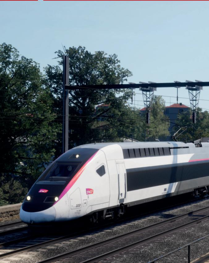
The Crocodile system is one of the oldest train safety systems operating in France. Status of upcoming signals is transmitted from electrical devices (named for their resemblance to a crocodile lying between the rails) that connect to on-board equipment located on the bottom of the train.
