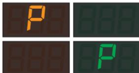
The yellow P is displayed to warn of a reduction to 160 km/h. It's followed by the green P when the reduction is enforced.
