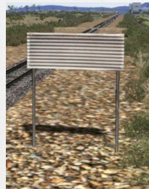
Warning board approximately 600 metres before a station. The driver sounds the loco's whistle/horn to warn the Station Master of an incoming train.
