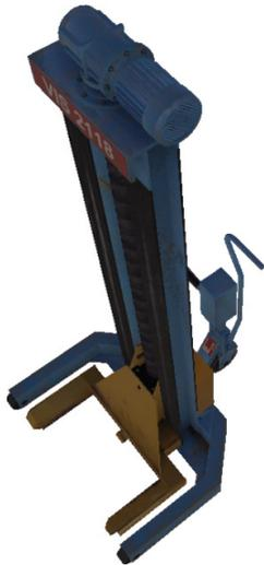
Using this tool, you can lift up the entire bus. To do this, all existing wheel engaging lifts must be pushed up to the bus. Once you have done this, the bus can be lifted and lowered in stages from any of the wheel engaging lifts. This helps you access different parts.
