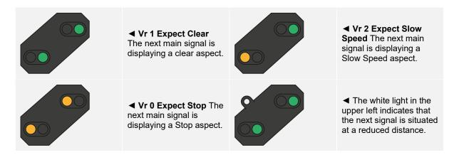
If Expect / Proceed at Reduced Speed is indicated without any white/yellow speed indicators, assume the maximum permitted speed is 40 km/h.
