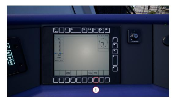
2. The display will present a representation of the trains in the consist and the destinations that are currently set, labelled 'ZUG 1', 'ZUG 2', etc. Press the '2' button (2) which is labelled 'Rout. Eing.' to set the destination.
